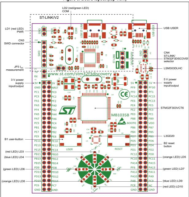
Figure 3. Board layout (top view)
