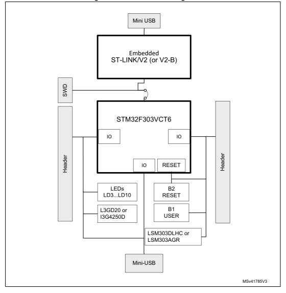
Figure 2. Hardware block diagram
