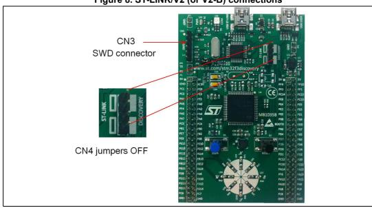
Figure 8. ST-LINK/V2 (or V2-B) connections
