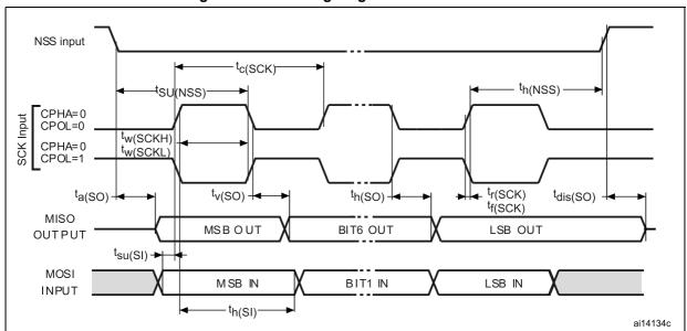
Figure 18. SPI timing diagram - slave mode and CPHA = 0
