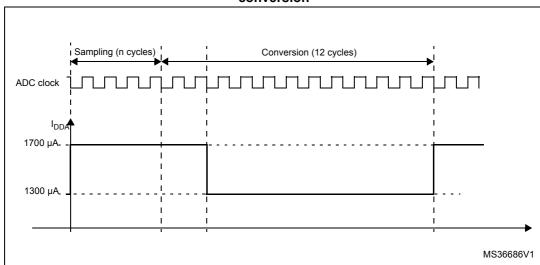
Figure 24. Maximum dynamic current consumption on V<sub>DDA</sub> supply pin during ADC conversion
