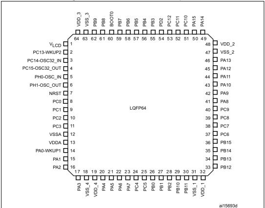
Figure 3. STM32L100RxxxA LQFP64 pinout
