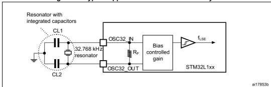
Figure 14. Typical application with a 32.768 kHz crystal
