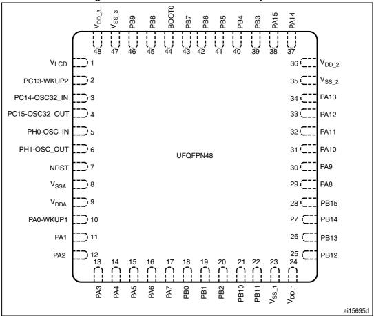
Figure 4. STM32L100C6xxA UFQFPN48 pinout
