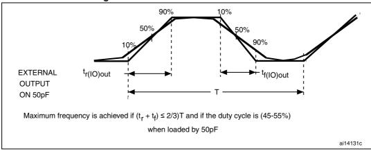
Figure 15. I/O AC characteristics definition
