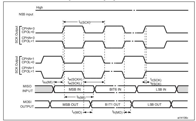
Figure 20. SPI timing diagram - master mode<sup>(1)</sup>
