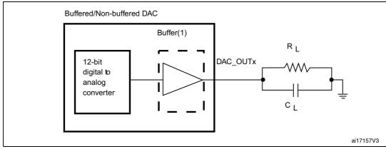
Figure 25. 12-bit buffered /non-buffered DAC
