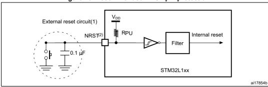
Figure 16. Recommended NRST pin protection
