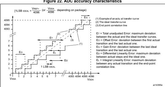
Figure 22. ADC accuracy characteristics
