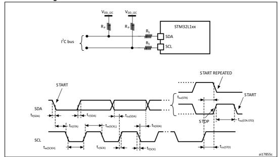
Figure 17. I<sup>2</sup>C bus AC waveforms and measurement circuit
