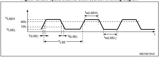
Figure 12. Low-speed external clock source AC timing diagram
