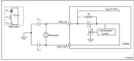
Figure 13. HSE oscillator circuit diagram
