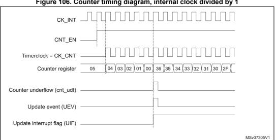
Figure 106. Counter timing diagram, internal clock divided by 1
