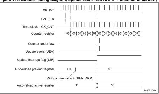
Figure 115. Counter timing diagram, Update event with ARPE=1 (counter underflow)
