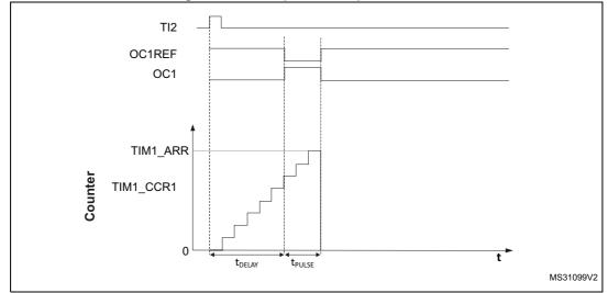
Figure 89. Example of one pulse mode.
