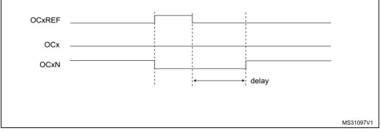
The dead-time delay is the same for each of the channels and is programmable with the DTG bits in the TIMx\_BDTR register. Refer to Section 14.4.18: TIM1 break and dead-time register (TIMx\_BDTR) for delay calculation.
