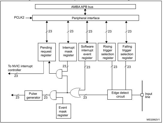
Figure 29. External interrupt/event controller block diagram
