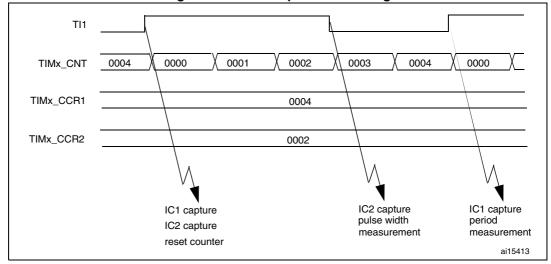
Figure 149. PWM input mode timing
