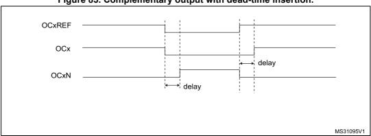
Figure 83. Complementary output with dead-time insertion.
