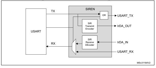
Figure 231. IrDA SIR ENDEC- block diagram
