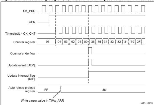
Figure 62. Counter timing diagram, update event when repetition counter is not used
