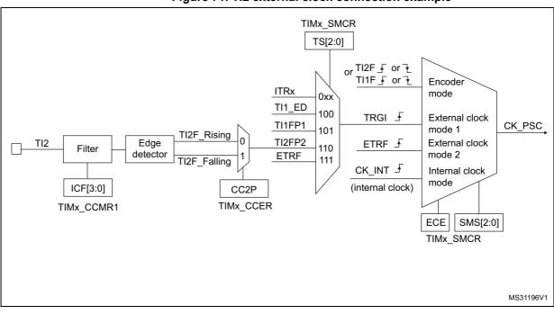
Figure 71. TI2 external clock connection example
