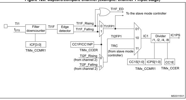
Figure 120. Capture/compare channel (example: channel 1 input stage)
