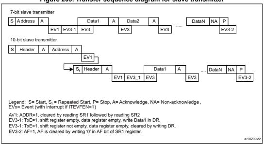
Figure 209. Transfer sequence diagram for slave transmitter
