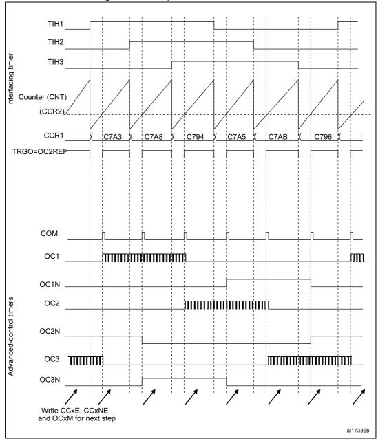
Figure 92. Example of Hall sensor interface
