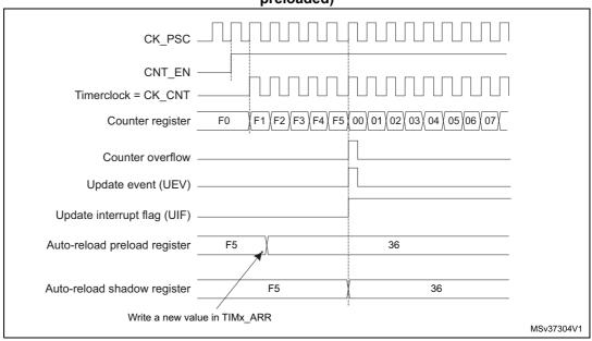
Figure 105. Counter timing diagram, Update event when ARPE=1 (TIMx\_ARR preloaded)
