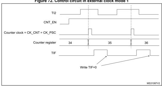
Figure 72. Control circuit in external clock mode 1
