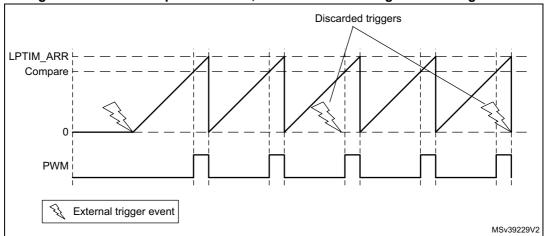
Figure 170. LPTIM output waveform, Continuous counting mode configuration
