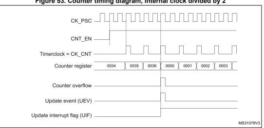
Figure 53. Counter timing diagram, internal clock divided by 2
