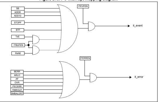
Figure 213. I<sup>2</sup>C interrupt mapping diagram
