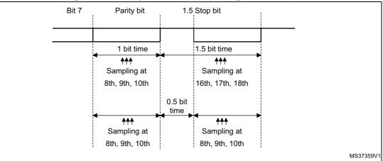
Figure 230. Parity error detection using the 1.5 stop bits
