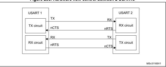
Figure 235. Hardware flow control between 2 USARTs
