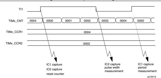
Figure 123. PWM input mode timing
