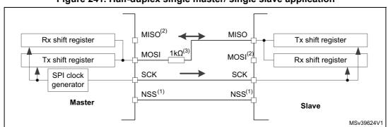
Figure 241. Half-duplex single master/ single slave application
