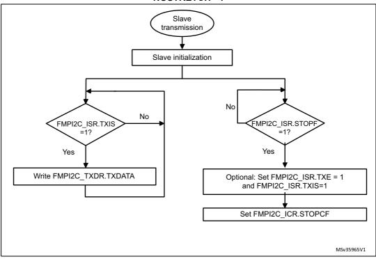
Figure 185. Transfer sequence flowchart for FMPI2C slave transmitter, NOSTRETCH= 1
