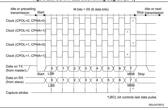
Figure 226. USART data clock timing diagram (M=0)
