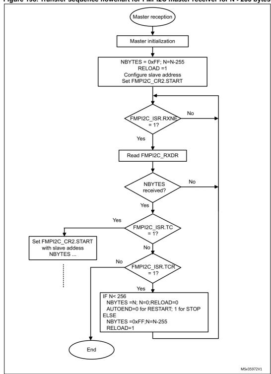
Figure 198. Transfer sequence flowchart for FMPI2C master receiver for N >255 bytes
