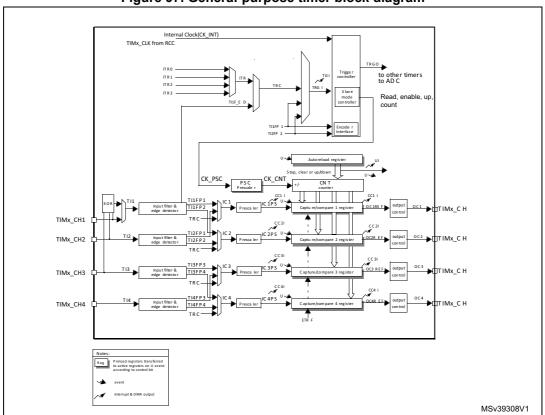
Figure 97. General-purpose timer block diagram
