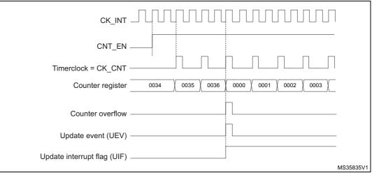
Figure 102. Counter timing diagram, internal clock divided by 4
