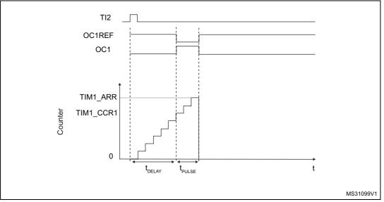
For example one may want to generate a positive pulse on OC1 with a length of  $t_{PULSE}$  and after a delay of  $t_{DELAY}$  as soon as a positive edge is detected on the TI2 input pin.
