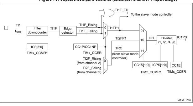
Figure 75. Capture/compare channel (example: channel 1 input stage)
