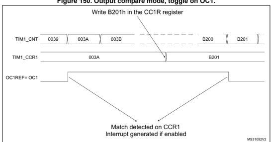
Figure 150. Output compare mode, toggle on OC1.
