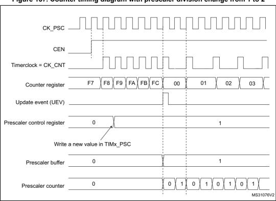
Figure 157. Counter timing diagram with prescaler division change from 1 to 2
