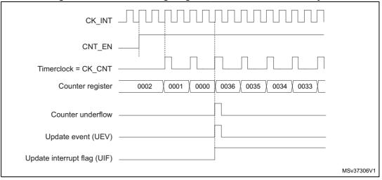
Figure 108. Counter timing diagram, internal clock divided by 4
