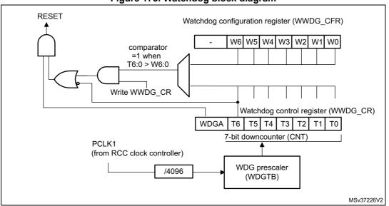
Figure 173. Watchdog block diagram
