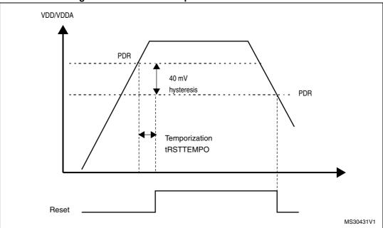
Figure 8. Power-on reset/power-down reset waveform
