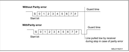
When connected to a Smartcard, the TX output of the USART drives a bidirectional line that
