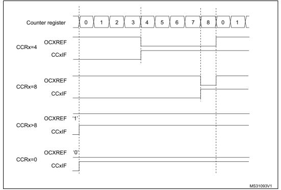
Figure 81. Edge-aligned PWM waveforms (ARR=8)
