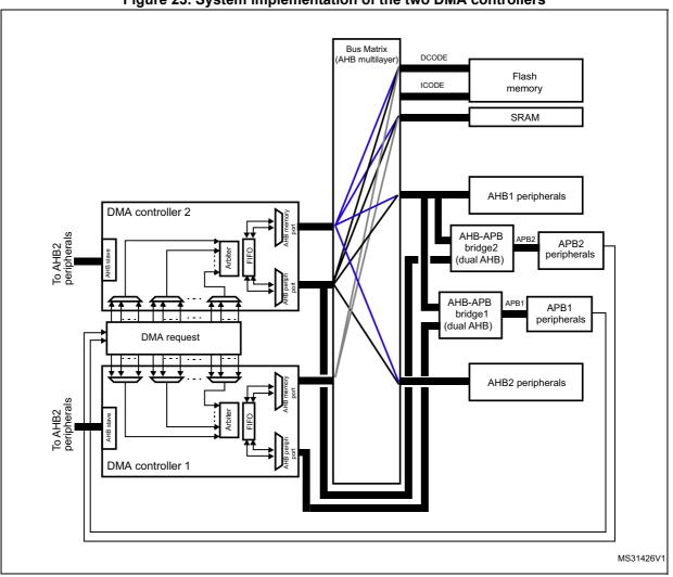
Figure 23. System implementation of the two DMA controllers
