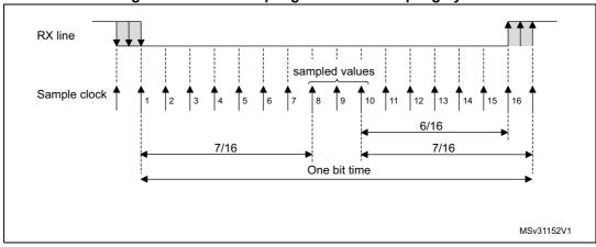
Figure 219. Data sampling when oversampling by 16
