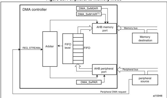
Figure 25. Peripheral-to-memory mode
