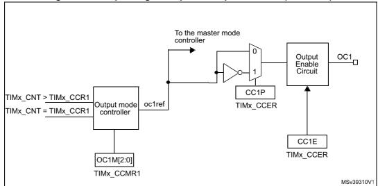
Figure 122. Output stage of capture/compare channel (channel 1)
