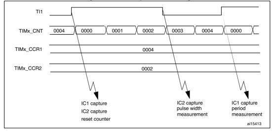
Figure 79. PWM input mode timing
