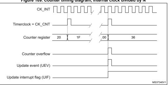
Figure 109. Counter timing diagram, internal clock divided by N
