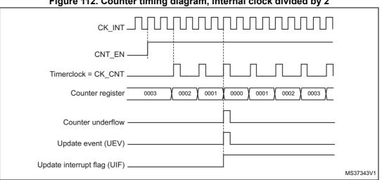
Figure 112. Counter timing diagram, internal clock divided by 2
