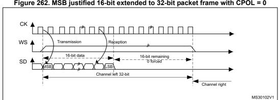
Figure 262. MSB justified 16-bit extended to 32-bit packet frame with CPOL = 0
