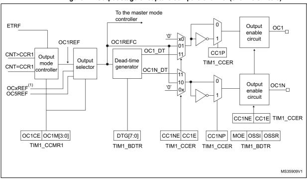
Figure 77. Output stage of capture/compare channel (channels 1 to 3)
