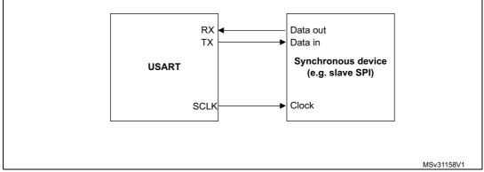
Figure 225. USART example of synchronous transmission
