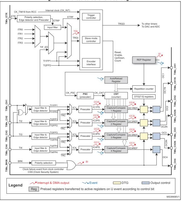
Figure 49. Advanced-control timer block diagram
