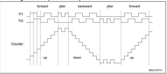
Figure 90. Example of counter operation in encoder interface mode.
