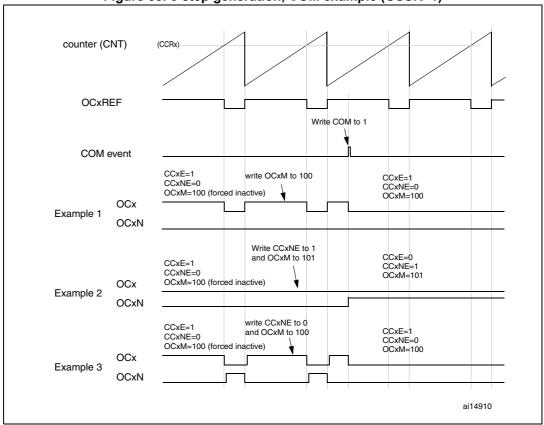
Figure 88. 6-step generation, COM example (OSSR=1)
