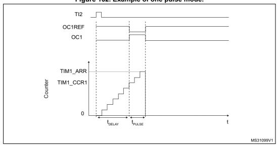
Figure 152. Example of one pulse mode.
