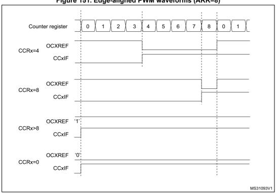
Figure 151. Edge-aligned PWM waveforms (ARR=8)
