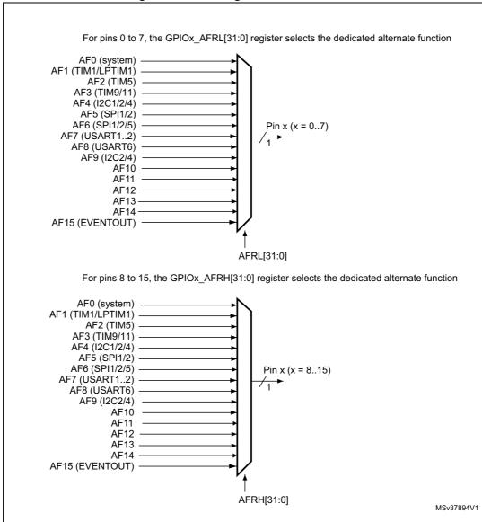
Figure 17. Selecting an alternate function
