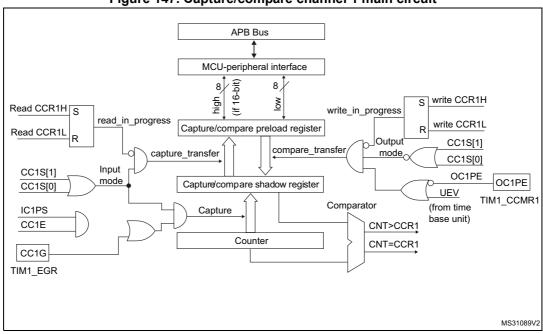
Figure 147. Capture/compare channel 1 main circuit
