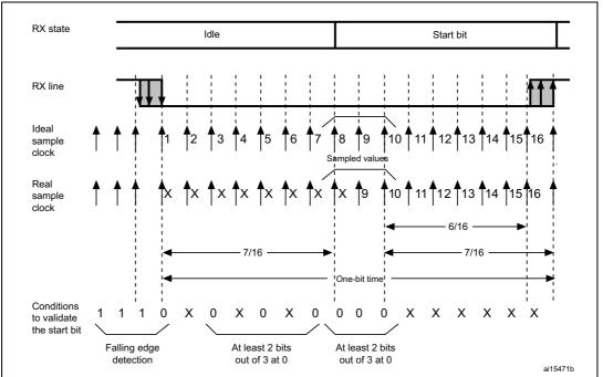
Figure 218. Start bit detection when oversampling by 16 or 8
