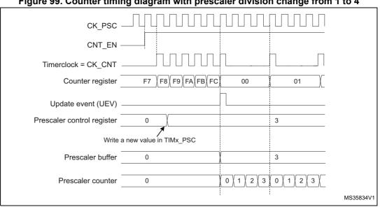
Figure 99. Counter timing diagram with prescaler division change from 1 to 4
