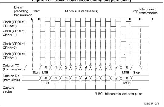
Figure 227. USART data clock timing diagram (M=1)
