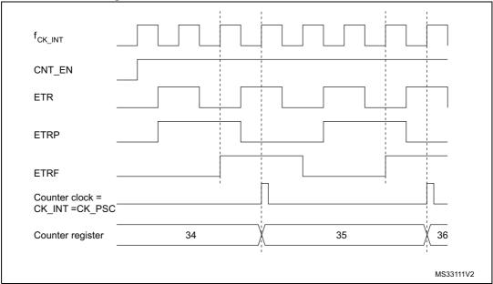
Figure 74. Control circuit in external clock mode 2
