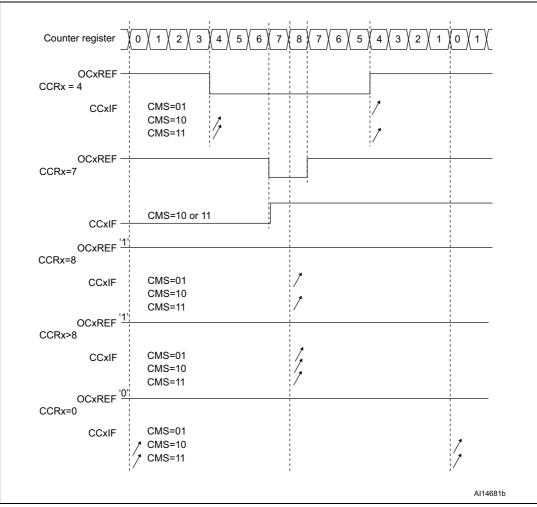
Figure 126. Center-aligned PWM waveforms (ARR=8)
