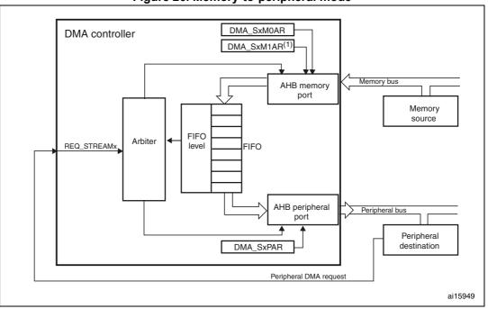
Figure 26. Memory-to-peripheral mode
