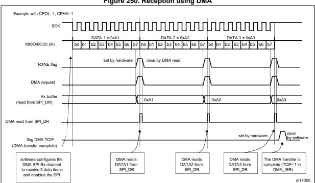
Figure 250. Reception using DMA
