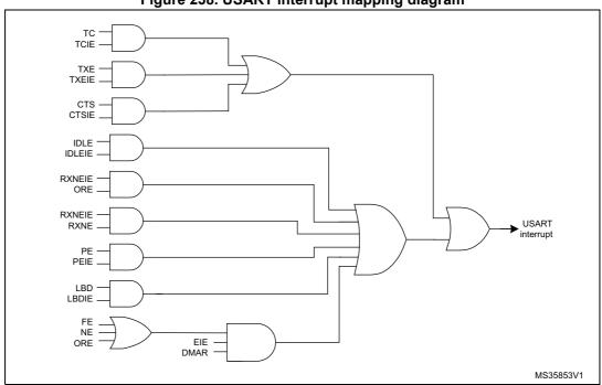
Figure 238. USART interrupt mapping diagram
