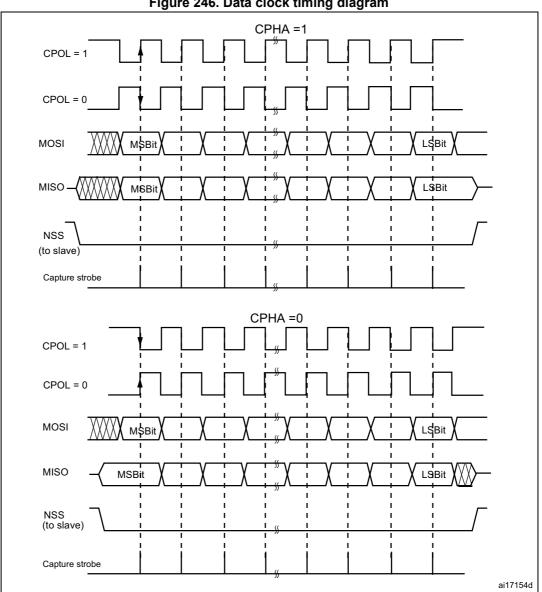
Figure 246. Data clock timing diagram
