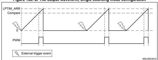
Figure 168. LPTIM output waveform, single counting mode configuration
