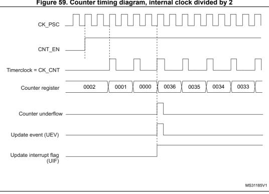
Figure 59. Counter timing diagram, internal clock divided by 2
