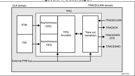
Figure 276. TPIU block diagram
