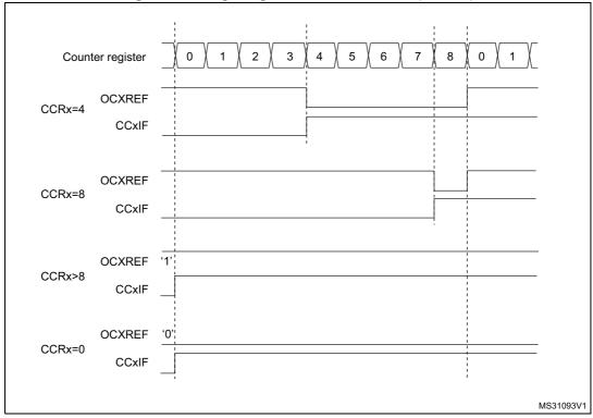
Figure 125. Edge-aligned PWM waveforms (ARR=8)
