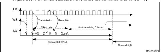
Figure 255.  $I^2$ S Philips standard waveforms (24-bit frame with CPOL = 0)
