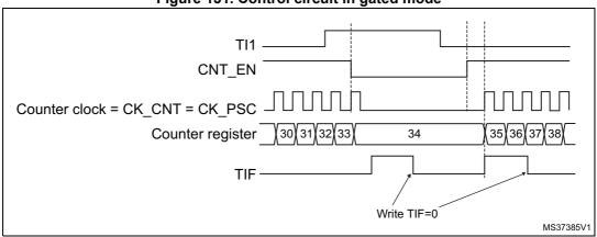
Figure 131. Control circuit in gated mode
