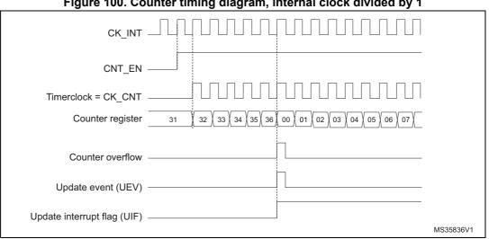
Figure 100. Counter timing diagram, internal clock divided by 1
