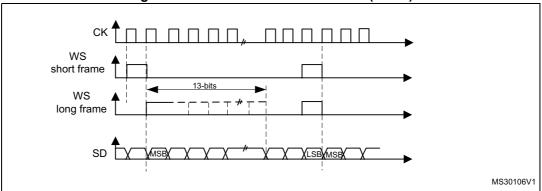
Figure 269. PCM standard waveforms (16-bit)
