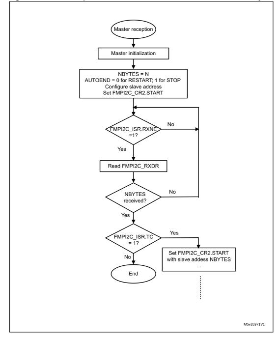
Figure 197. Transfer sequence flowchart for FMPI2C master receiver for N≤255 bytes
