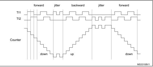
Figure 91. Example of encoder interface mode with TI1FP1 polarity inverted.
