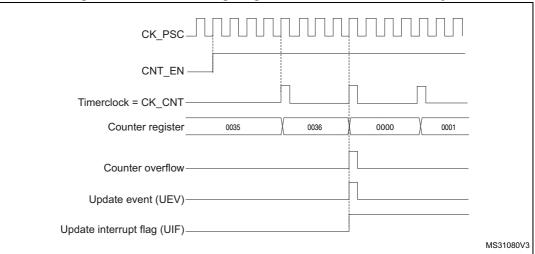
Figure 55. Counter timing diagram, internal clock divided by N
