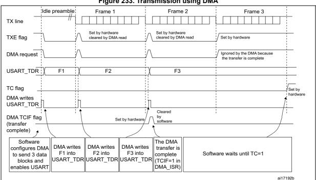
Figure 233. Transmission using DMA
