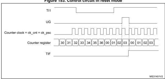
Figure 153. Control circuit in reset mode
