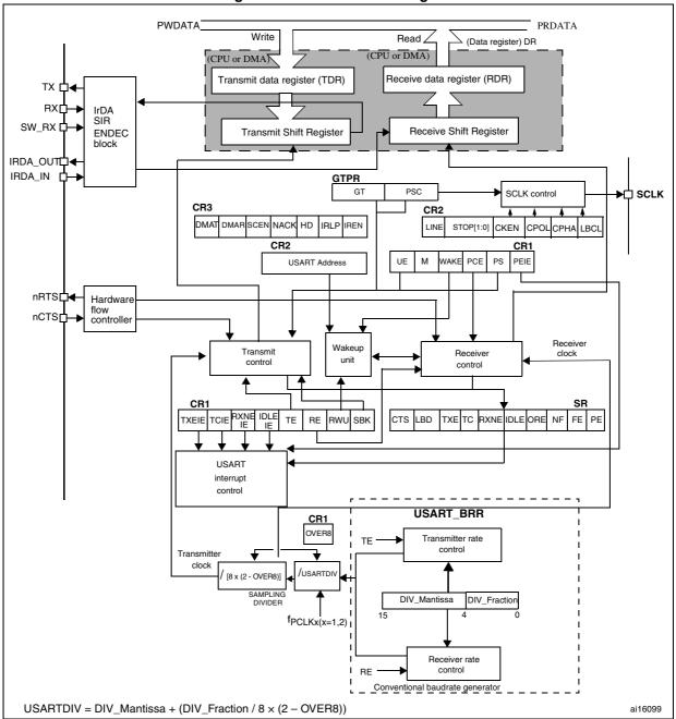
Figure 214. USART block diagram
