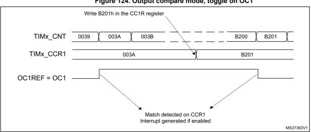
Figure 124. Output compare mode, toggle on OC1
