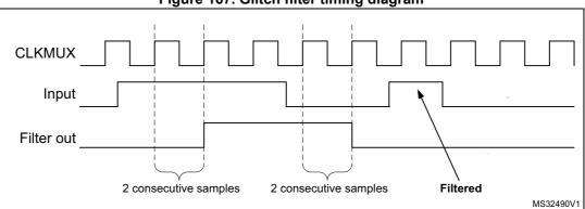
Figure 167. Glitch filter timing diagram
