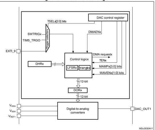
Figure 40. DAC channel block diagram
