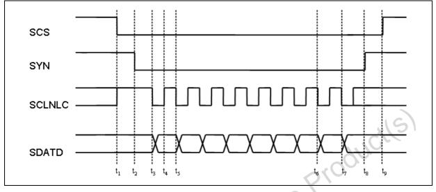
Figure 21. Timing for writing configuration and mode bits
