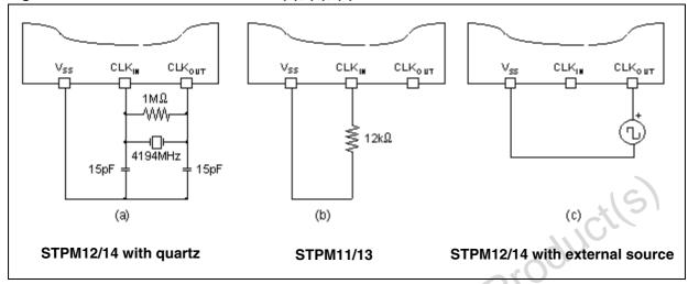
Figure 18. Different oscillator circuits (a); (b); (c)
