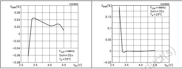
Figure 9. Power supply AC rejection vs.  $V_{CC}$  Figure 10. Power supply DC rejection vs.  $V_{CC}$
