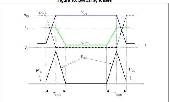
Figure 16. Switching losses
