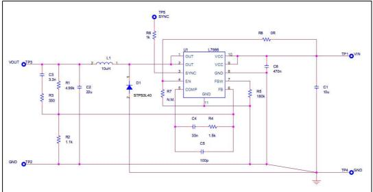
Figure 18. Demonstration board application circuit
