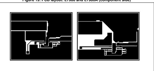
Figure 19. PCB layout: L7986 and L7986A (component side)
