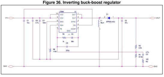
The GND pin of the device is connected to the output voltage so, given the output voltage, the input voltage range is limited by the maximum voltage the device can withstand across VCC and GND (38 V). Therefore, if the output is -5 V the input voltage can range from 4.5 V to 33 V.
