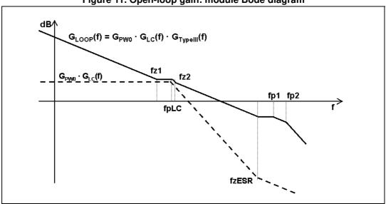
Figure 11. Open-loop gain: module Bode diagram
