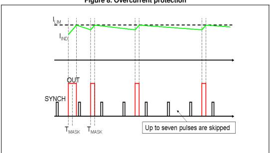
Figure 8. Overcurrent protection
