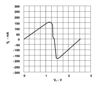
Figure 9. Bus-Hold Current With V<sub>CC</sub> = 3 V and V<sub>I</sub> Sweep From 0 V to 3 V
