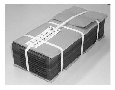
Figure 5. Example of Trays Stacked and Bound
