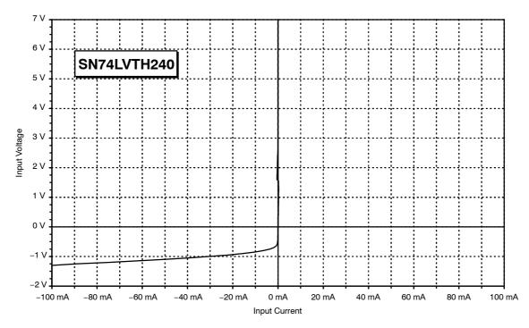
Figure 7. Input Characteristic of the SN74LVTHxxx Series
