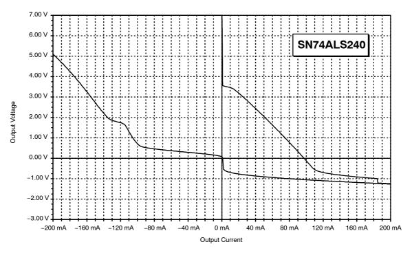
Figure 23. Output Characteristic of the SN74ALS240
