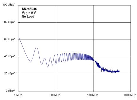
Figure 54. SN74F245 Spectrum of the Supply Current (output unloaded)
