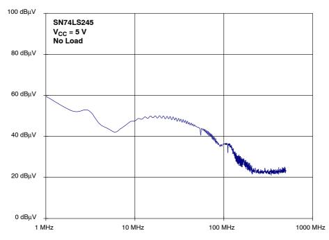
Figure 62. SN74LS245 Spectrum of the Supply Current (output unloaded)
