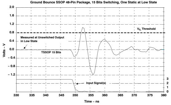
Figure 7. Measured Simultaneous-Switching Ground Bounce, SSOP 48-Pin Package
