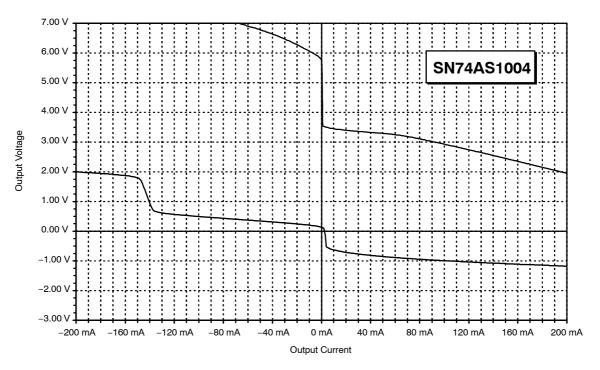
Figure 27. Output Characteristic of the SN74AS1004
