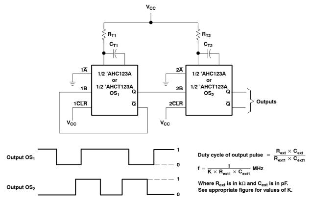
Figure 11. Low-Power Pulse Generator
