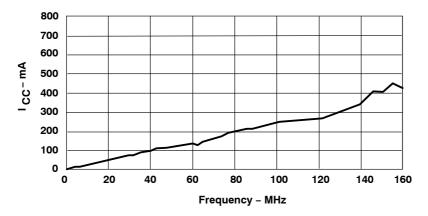
Figure 17. I<sub>CC</sub> vs Frequency (16 Outputs Switching)
