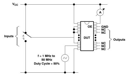
Figure 2. Power Consumption vs Frequency Measurement Setup
