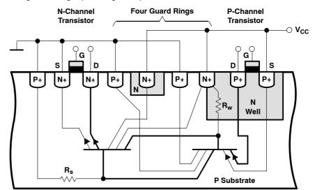
Figure 3. Guard Rings in a CMOS Circuit
