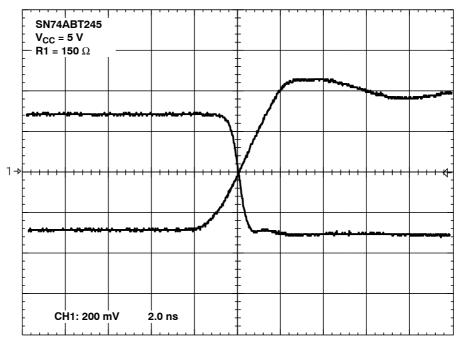
Figure 16. SN74ABT245 Waveform at the Output
