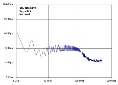
Figure 50. SN74BCT245 Spectrum of the Supply Current (output unloaded)
