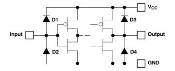
Figure 11. ESD-Protection Circuits Using Diodes
