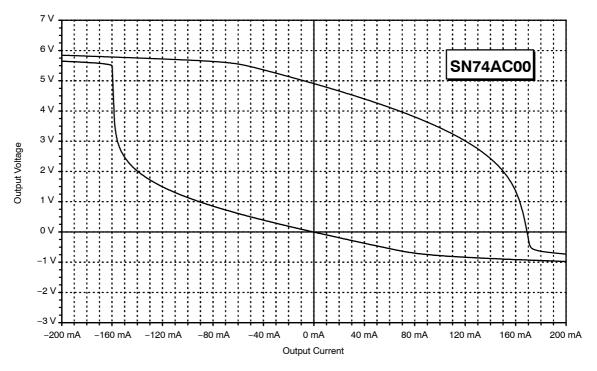
Figure 35. Output Characteristic of the SN74AC00
