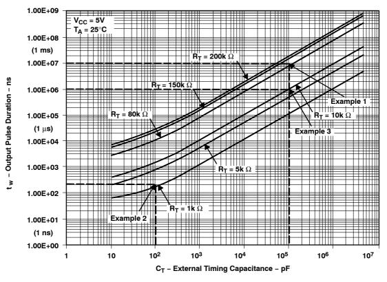
Figure 3. Output Pulse Duration vs External Timing Capacitance
