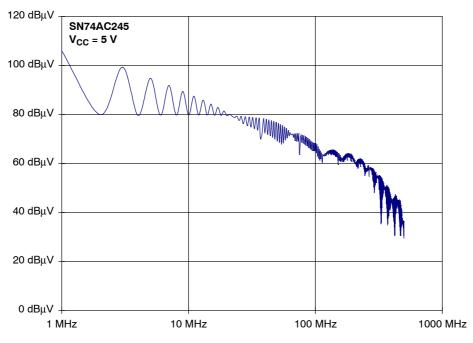
Figure 8. Spectrum of the Output Signal of an AC Circuit
