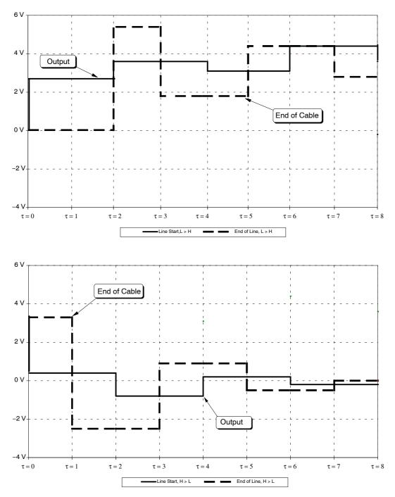
Figure 24. Diagram of Line Reflections for the SN74ALVTH16244
