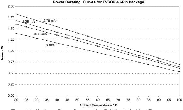
Figure 23. Maximum Power Consumption Relative to Ambient Temperature,  $T_J = 150^{\circ}C$ , TVSOP 48-Pin Package
