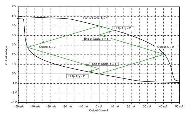
Figure 45. Bergeron Diagram for the SN74AHC240
