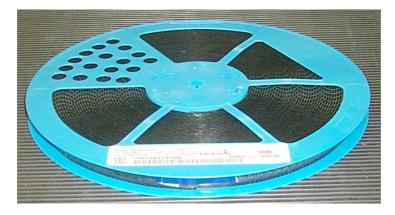
Figure 3. Reel With Carrier Tape
