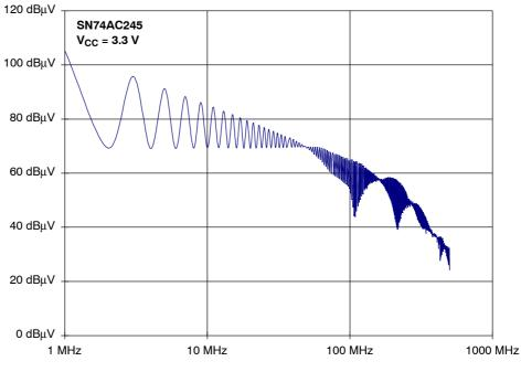
Figure 29. SN74AC245 Spectrum of the Output Signal
