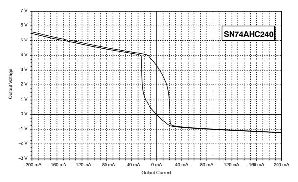
Figure 11. Output Characteristics of the SN74AHC240
