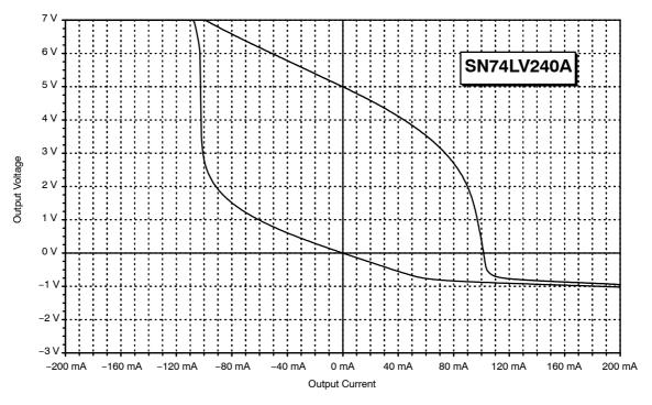
Figure 43. Output Characteristic of the SN74LV240A
