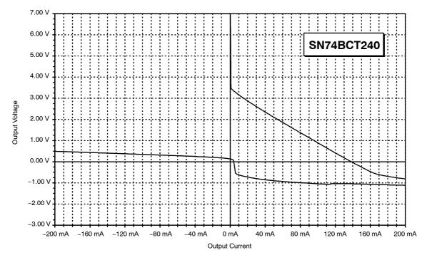
Figure 37. Output Characteristic of the SN74BCT240
