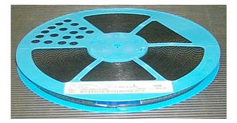
Figure 14. Loaded Reel (Not Moisture Sensitive)
