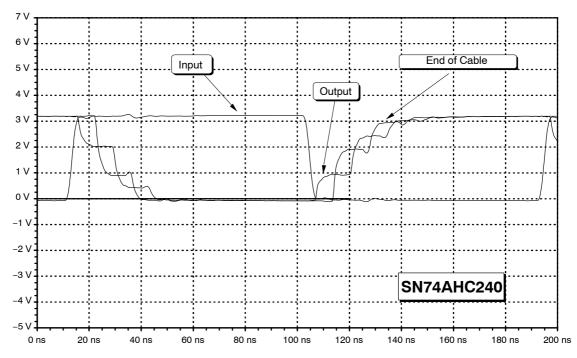
Figure 26. Output Waveforms of the SN74AHC240
