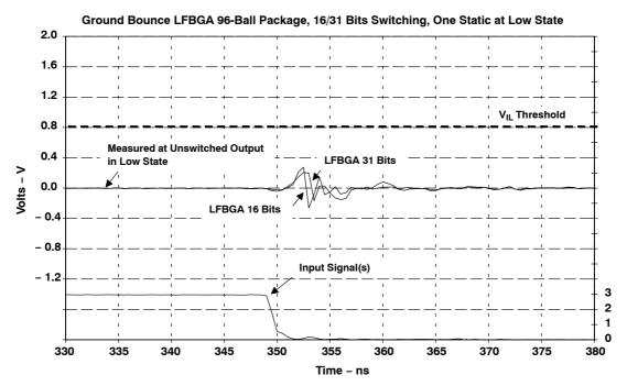
Figure 10. Measured Simultaneous-Switching Ground Bounce, LFBGA 96 Ball
