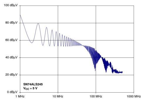
Figure 43. SN74ALS245 Spectrum of the Supply Current (output loaded)
