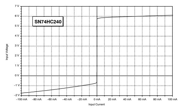
Figure 7. Input Characteristic of the SN74HCxxx Series
