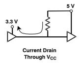
Figure 14. 3.3-V Driver Pulled to a Higher V<sub>CC</sub>
