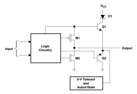
Figure 3. ALVT Output Circuit
