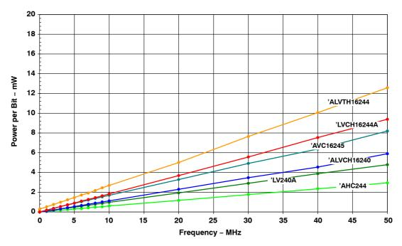
Figure 4. Power Consumption at 2.5-V  $V_{CC}$
