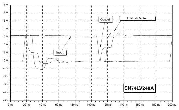
Figure 29. Output Waveforms of the SN74LV240A
