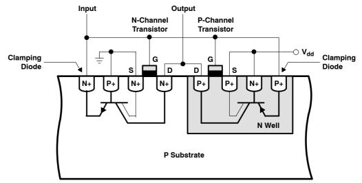
Figure 17. Parasitic Transistors in CMOS Circuits
