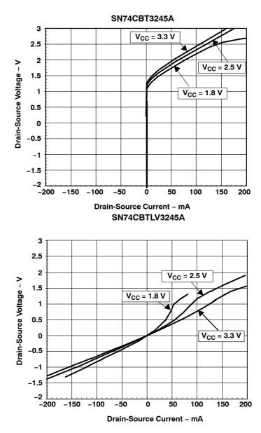
Figure 9. High-State ron of CBT3245A and CBTLV3245A at Different Supply Voltages
