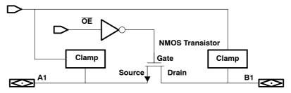
Figure 4. Basic NMOS Switch With Active-Clamp Pullup Circuits
