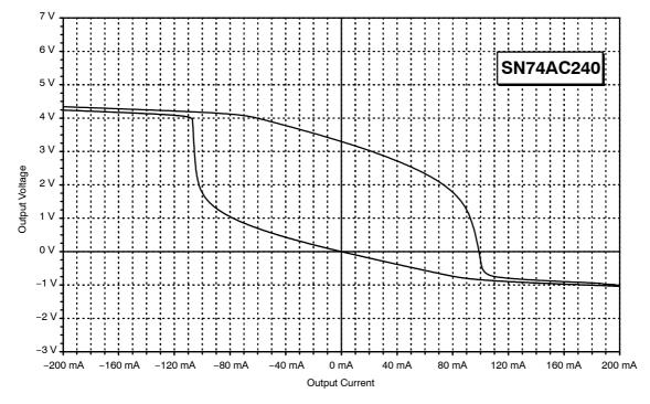
Figure 13. Output Characteristics of the SN74AC240
