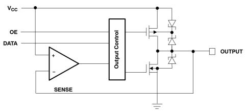
Figure 9. Simplified Output Stage of ALVT Devices
