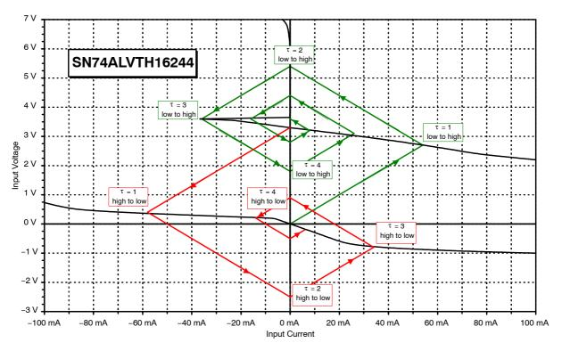
Figure 23. Bergeron Diagram for the SN74ALVTH16244
