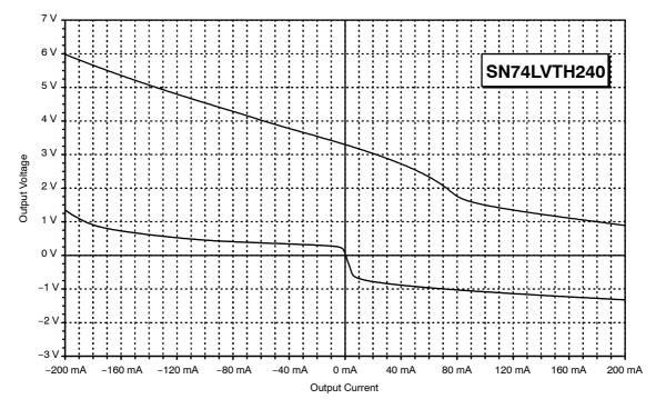
Figure 19. Output Characteristics of the SN74LVTH240
