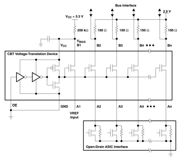
Figure 4. Typical Application of CBT as a Voltage-Translation Device
