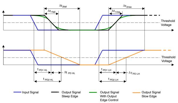
Figure 3. Influence of Slew Rate on Propagation Delay Time and the Principle Behind OEC
