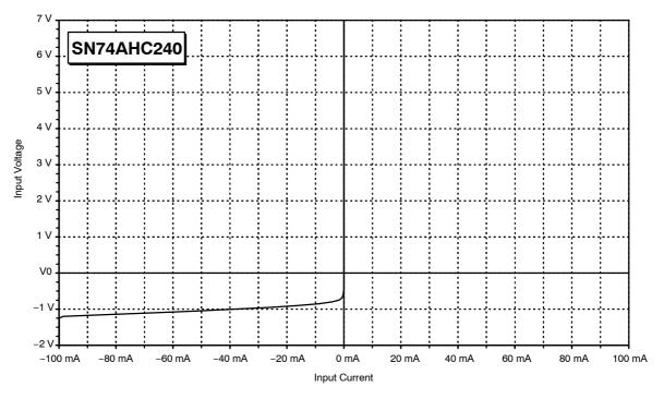
Figure 1. Input Characteristic of the SN74AHCxxx Series
