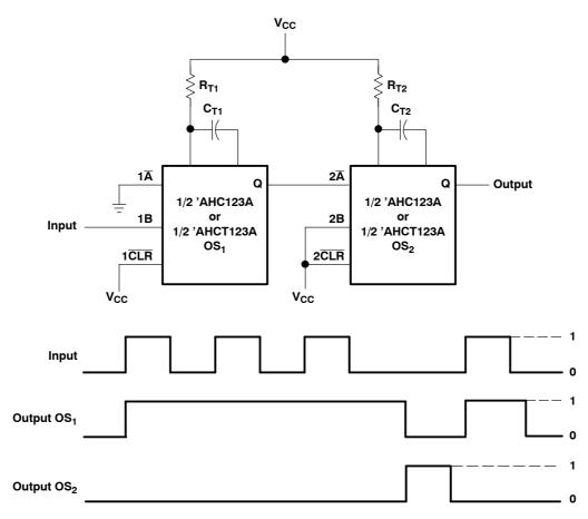
Figure 10. Missing-Pulse Detector
