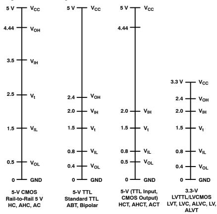
Figure 3. Comparison of Switching Standards
