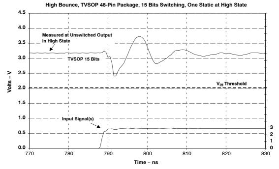
Figure 13. Measured Simultaneous-Switching High Bounce, TVSOP 48-Pin Package
