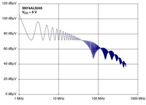
Figure 41. SN74ALS245 Spectrum of the Output Signal
