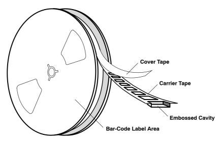
Figure 7. Tape-and-Reel Packing
