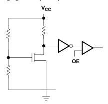
Figure 10. Power-Up Control Circuit
