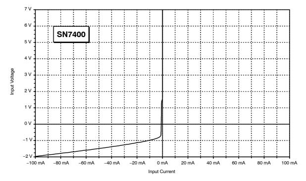
Figure 1. Input Characteristic of the SN74xxx Series
