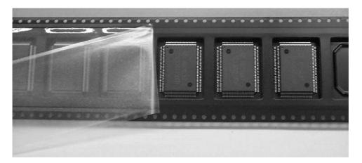
Figure 9. Rectangular QFP Package Properly Oriented in Carrier Tape
