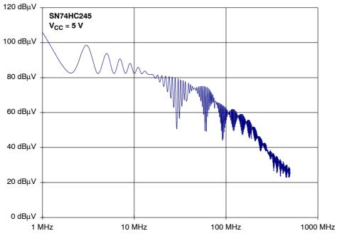
Figure 57. SN74HC245 Spectrum of the Output Signal
