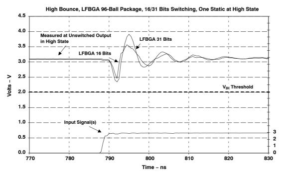
Figure 14. Measured Simultaneous-Switching High Bounce, LFBGA 96 Ball
