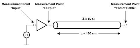
Figure 44. Measurement Setup for the Bergeron Method
