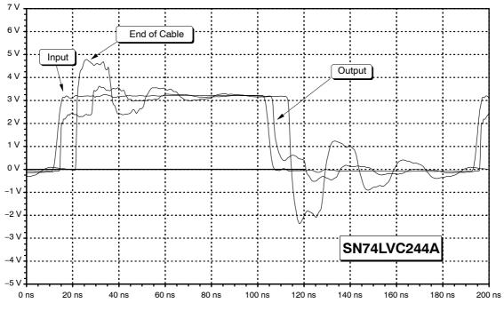
Figure 30. Output Waveforms of the SN74LVC244A
