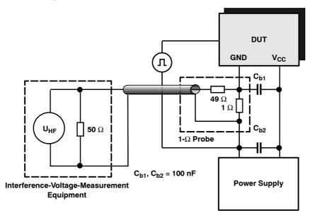
Figure 4. Measurement of the Supply Current
