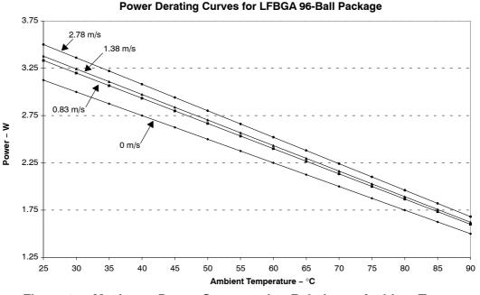
Figure 24. Maximum Power Consumption Relative to Ambient Temperature,  $T_J = 150^{\circ}C$ , LFBGA 96 Ball
