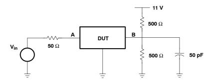
Figure 5. Test Setup for the Undershoot Test
