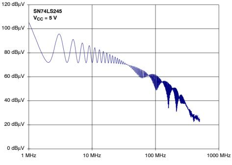
Figure 61. SN74LS245 Spectrum of the Output Signal
