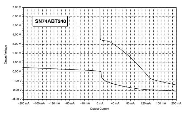
Figure 39. Output Characteristic of the SN74ABT240
