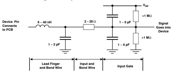
Figure 11. MOS Buffer Simplified Schematic
