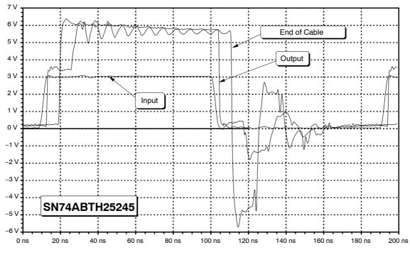
Figure 75. Output Waveforms of the SN74ABTH25245
