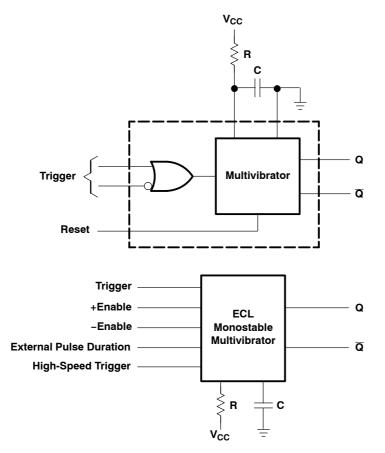
Figure A-1. One-Shot Monostable Multivibrator and Function Block Diagram
