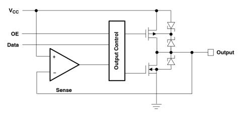
Figure 6. Simplified Auto3-State Output Stage of ALVT Devices
