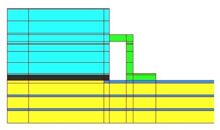
Figure 4. Cross Section of 20-Pin SOIC Package on 2s2p PCB
