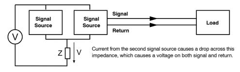
Common-mode noise is the noise voltage that travels down both the signal and return caused by a voltage drop across a shared impedance. Ground bounce on outputs is an example of common-mode noise.
