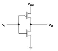
Figure 1. ALVT Input Structure
