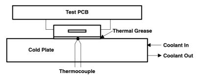
Figure 2.  $\theta_{\text{JC}}$  Laboratory Measurement Method
