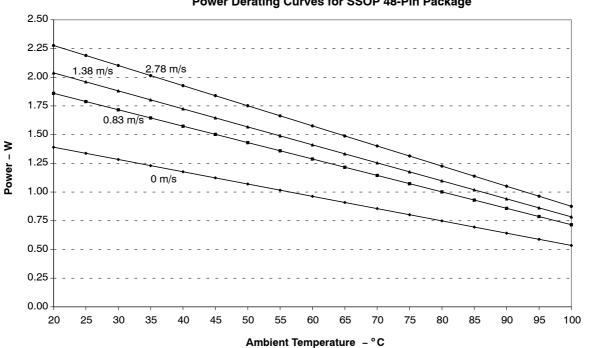
Figure 21. Maximum Power Consumption Relative to Ambient Temperature, T<sub>J</sub> = 150°C, SSOP 48-Pin Package
