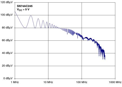
Figure 25. SN74AC245 Spectrum of the Output Signal
