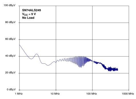
Figure 42. SN74ALS245 Spectrum of the Supply Current (output unloaded)
