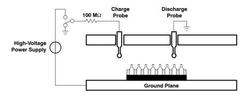
Figure 10. Charged-Device Model Test Setup
