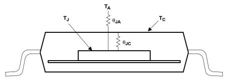
Figure 1. IC Package Thermal Metrics
