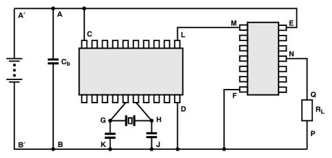
Figure 2. Current Loops on a Circuit Board
