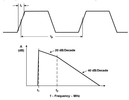
Figure 5. Spectrum of a Digital Signal
