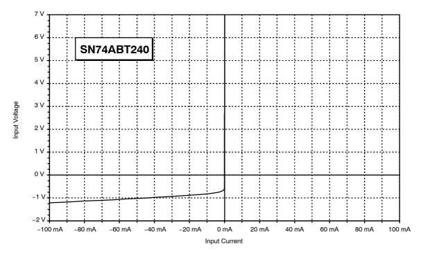
Figure 11. Input Characteristic of the SN74ABTxxx Series
