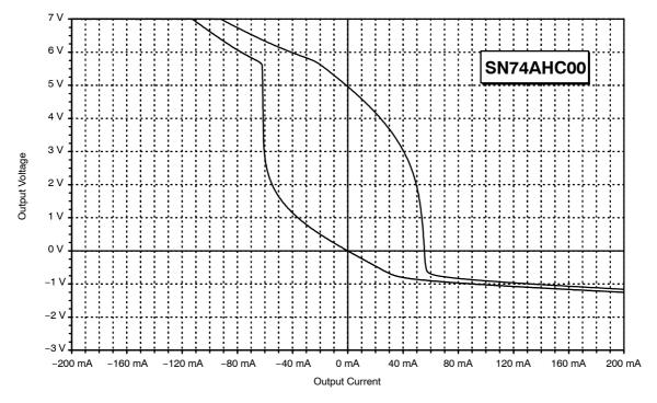
Figure 33. Output Characteristic of the SN74AHC00
