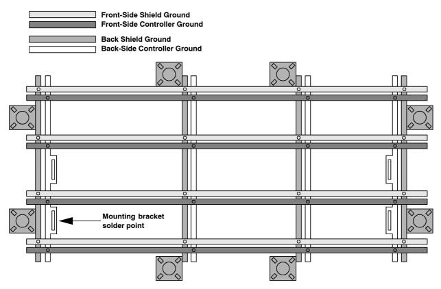
Figure 12. Front-Panel Gridding to Form Two Ground Planes
