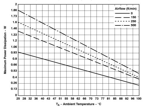
Figure 5. Derating Curves for 16-Pin DW SOIC Package
