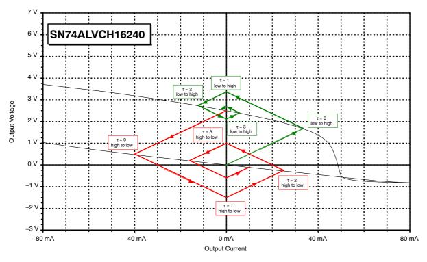
Figure 16. Bergeron Diagram for the SN74ALVCH16240
