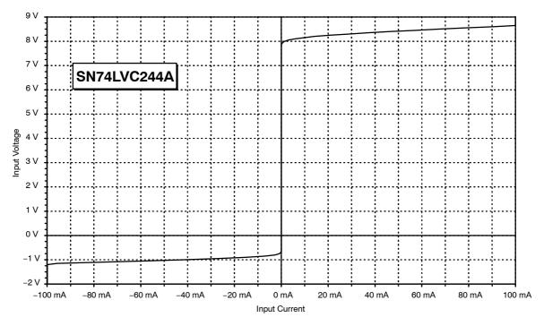
Figure 3. Input Characteristic of the SN74LVCxxx Series
