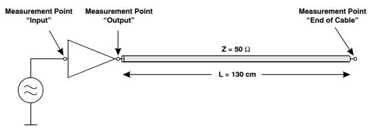
Figure 22. Measurement Setup for the Bergeron Method
