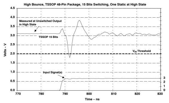
Figure 12. Measured Simultaneous-Switching High Bounce, TSSOP 48-Pin Package
