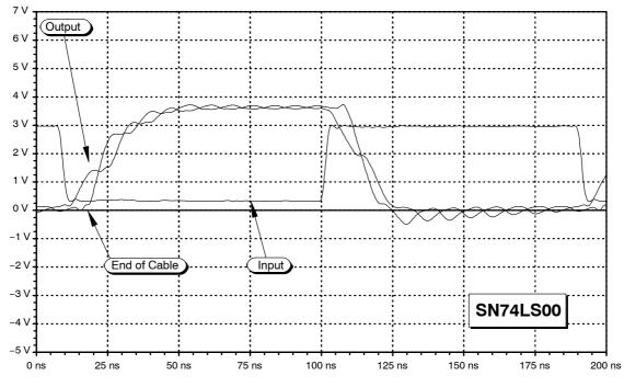
Figure 51. Output Waveforms of the SN74LS00
