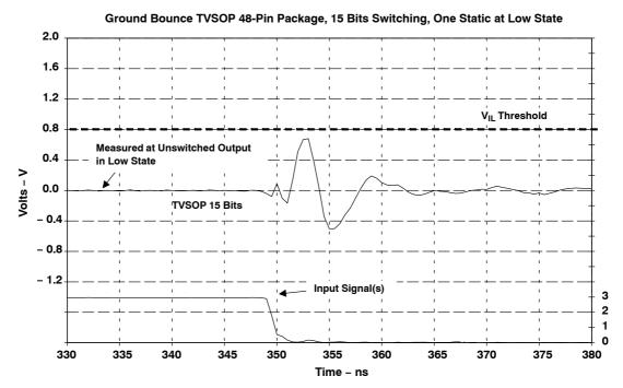
Figure 9. Measured Simultaneous-Switching Ground Bounce, TVSOP 48-Pin Package
