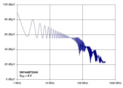
Figure 23. SN74ABT2245 Spectrum of the Supply Current (output loaded)
