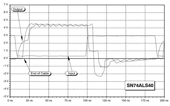
Figure 58. Output Waveforms of the SN74ALS40
