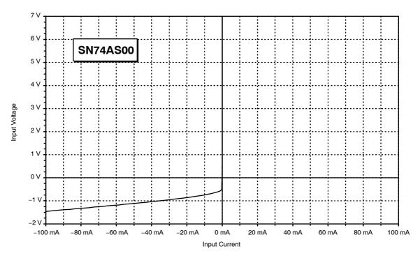
Figure 5. Input Characteristic of the SN74ASxxx Series
