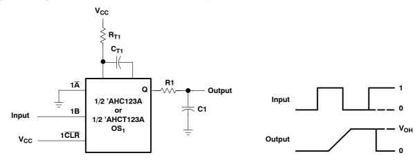
Figure 14. Frequency-Discriminator Circuit
