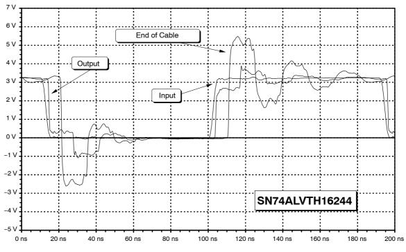
Figure 34. Output Waveforms of the SN74ALVTH16244
