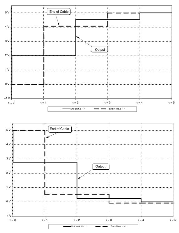
Figure 46. Diagram of Line Reflections for the SN74AHC240
