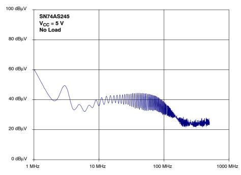
Figure 46. SN74AS245 Spectrum of the Supply Current (output unloaded)
