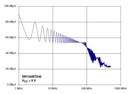
Figure 19. SN74ABT245 Spectrum of the Supply Current (output loaded)
