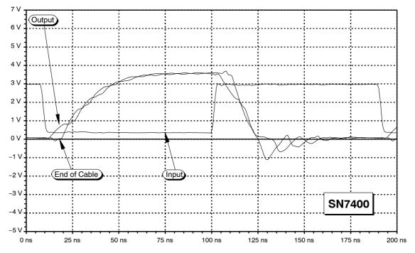
Figure 49. Output Waveforms of the SN7400
