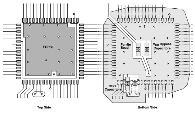
Figure 4. Microcomputer Ground
