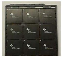
Figure 6. JEDEC Tray With Properly Arranged Units
