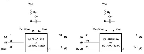
Figure 2. Timing Component Connections
