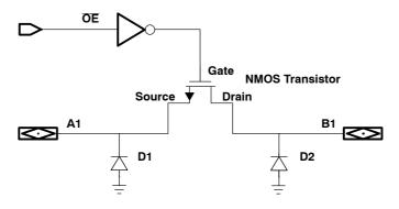
Figure 1. Basic NMOS-Transistor Bus Switch
