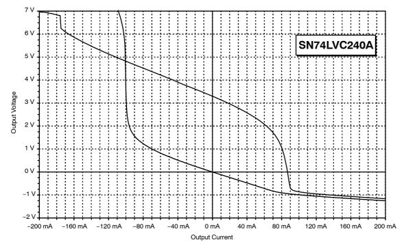
Figure 17. Output Characteristics of the SN74LVC240A
