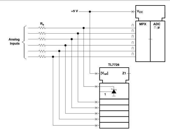
Figure 19. A/D Converter With Limitation of the Input Voltage
