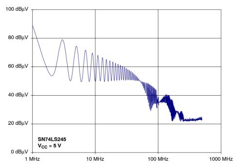
Figure 63. SN74LS245 Spectrum of the Supply Current (output loaded)
