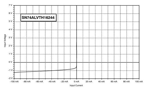
Figure 8. Input Characteristic of the SN74ALVTHxxx Series
