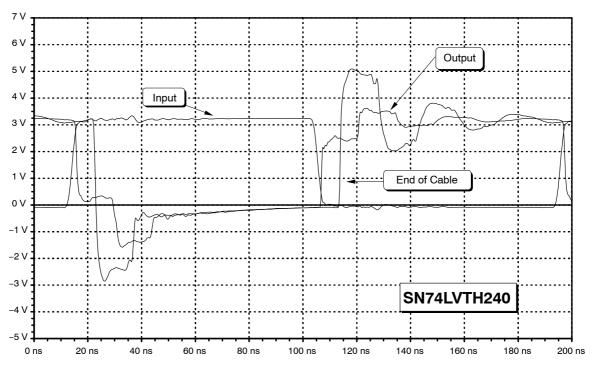
Figure 33. Output Waveforms of the SN74LVTH240
