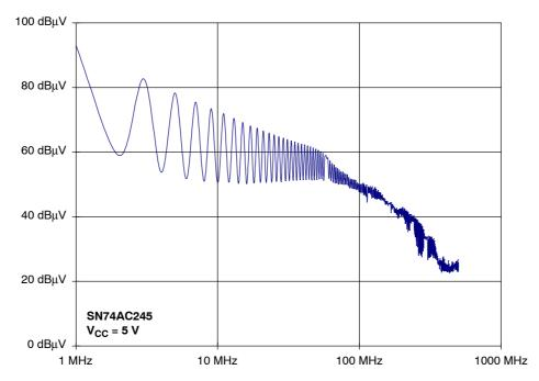
Figure 27. SN74AC245 Spectrum of the Supply Current (output loaded)
