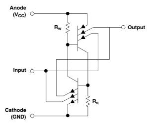
Figure 2. Parasitic Thyristor in a CMOS Circuit
