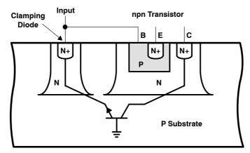
Figure 15. Parasitic Transistors in Bipolar Circuits
