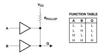
Figure 17. Wired Links Using Open-Drain Connections
