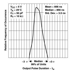
Figure 8. Distribution of Units vs Output Pulse Duration
