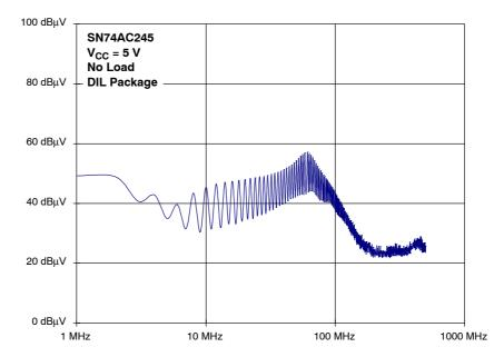
Figure 13. Frequency Spectrum of the Supply Current of an Unloaded AC Circuit (DIL package)
