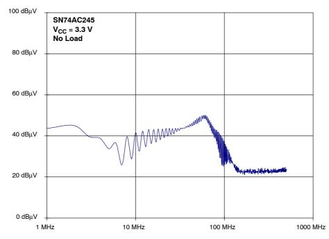
Figure 30. SN74AC245 Spectrum of the Supply Current (output unloaded)
