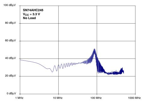
Figure 38. SN74AHC245 Spectrum of the Supply Current (output unloaded)
