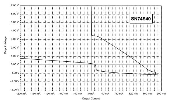
Figure 19. Output Characteristic of the SN74S40
