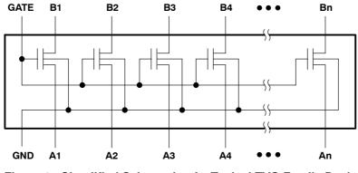
Figure 2. Simplified Schematic of a Typical TVC-Family Device
