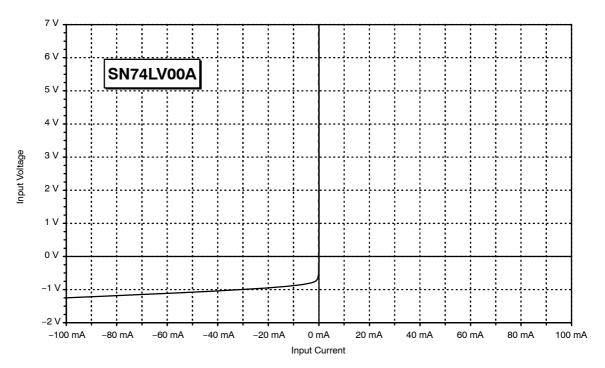
Figure 12. Input Characteristic of the SN74LVxxx Series
