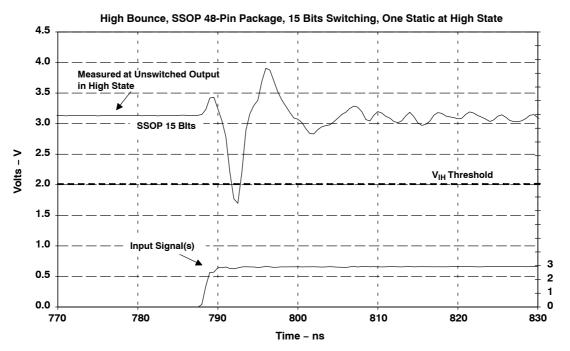
Figure 11. Measured Simultaneous-Switching High Bounce, SSOP 48-Pin Package
