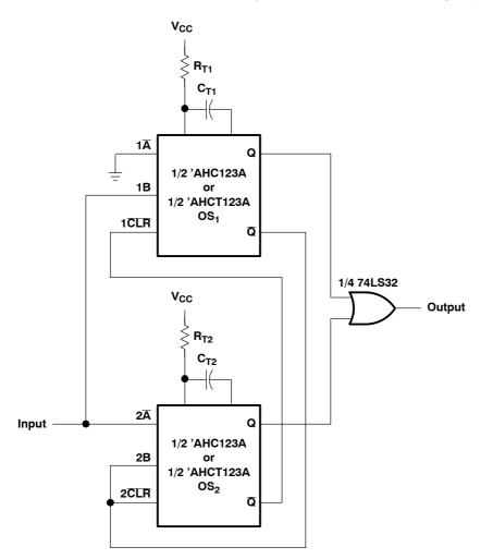
Figure 12. Negative- or Positive-Edge-Triggered One-Shot Multivibrator
