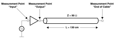
Figure 48. Measurement Setup for the Bergeron Method
