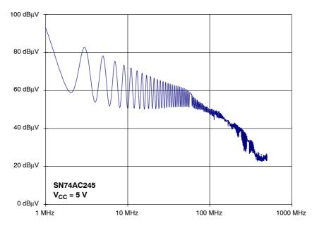
Figure 15. Frequency Spectrum of the Supply Current of a Loaded AC Circuit
