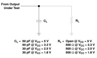
Figure 11. Test Conditions for Measuring Propagation Delay Time
