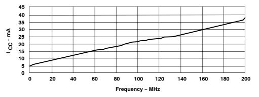
Figure 16. I<sub>CC</sub> vs Frequency (Single-Output Switching Enabled)
