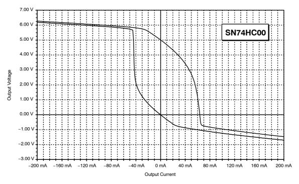
Figure 31. Output Characteristic of the SN74HC00
