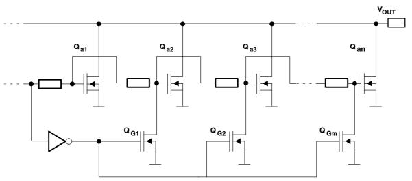
Figure 4. Basic Structure of the OEC Output Stage
