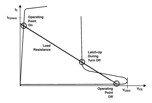
Figure 6. Output Characteristics With Load Resistor
