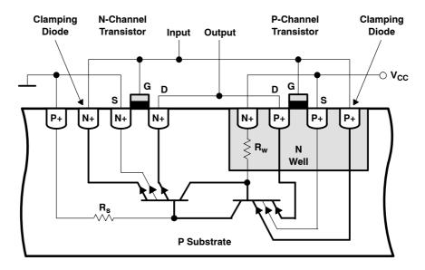
Figure 1. Parasitic Transistors in a CMOS Circuit
