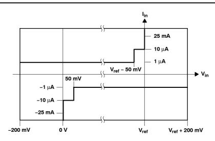
Figure 18. Characteristics of Voltage Limiter TL7726
