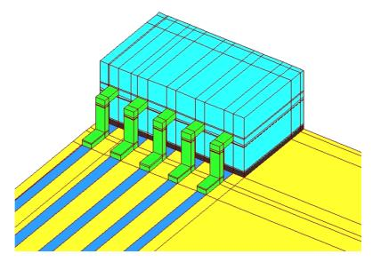
Figure 3. One-Quarter Package Model of 20-Pin SOIC Package
