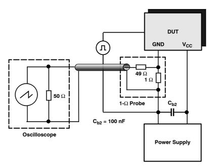
Figure 9. Test Circuit for Determination of Current Spikes
