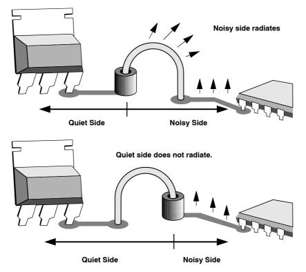
Figure 9. Ferrite-Bead Placement Closest to the Noise Source
