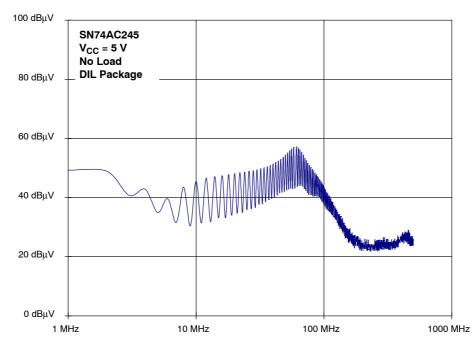
Figure 26. SN74AC245 Spectrum of the Supply Current (output unloaded)
