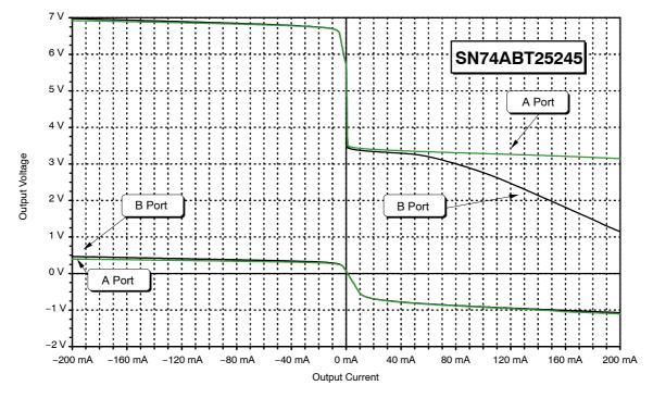
Figure 41. Output Characteristic of the SN74ABT25245
