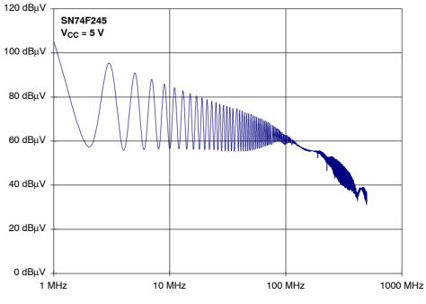
Figure 53. SN74F245 Spectrum of the Output Signal
