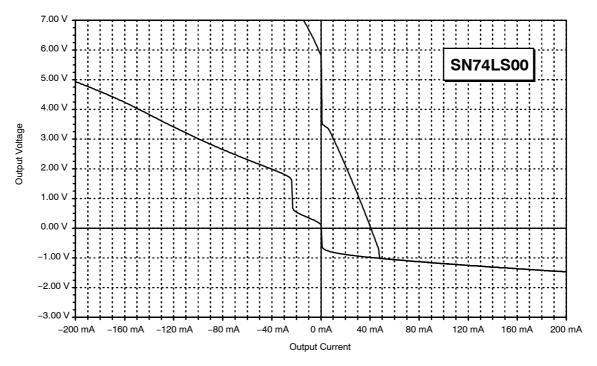
Figure 15. Output Characteristic of the SN74LS00
