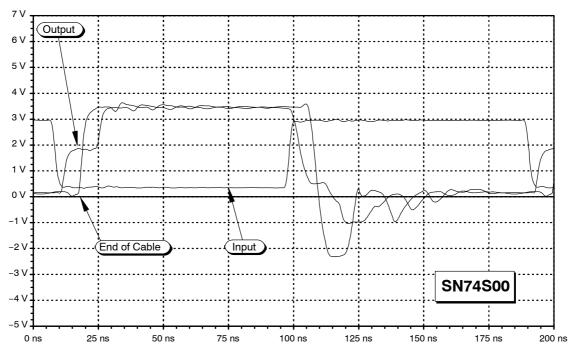
Figure 54. Output Waveforms of the SN74S00
