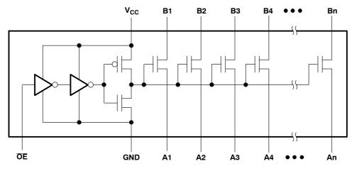
Figure 3. Simplified Schematic of a Typical CBT-Family Device
