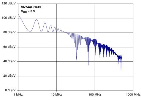
Figure 33. SN74AHC245 Spectrum of the Output Signal
