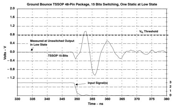
Figure 8. Measured Simultaneous-Switching Ground Bounce, TSSOP 48-Pin Package
