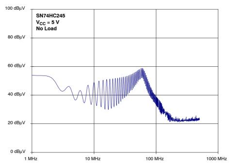
Figure 58. SN74HC245 Spectrum of the Supply Current (output unloaded)
