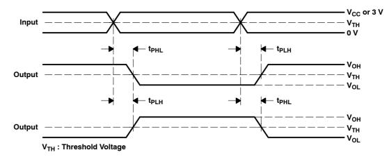
Figure 12. Propagation Delay Times of Inverting and Noninverting Outputs
