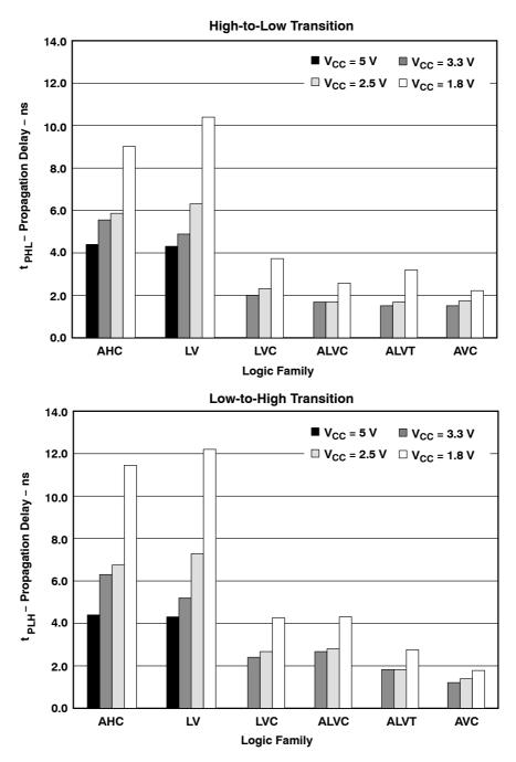
Figure 13. Typical Propagation Delays at Different Supply Voltages
