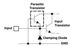
Figure 16. Input Circuit With Parasitic Transistor
