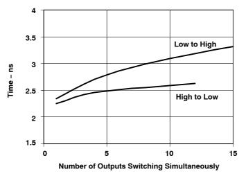
Figure 15.  $t_{pd}$  vs Simultaneous Switching,  $V_{CC}$  = 3.3 V and 50 pF
