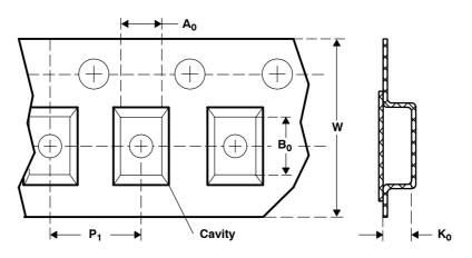
Figure 8. Carrier-Tape Dimensions
