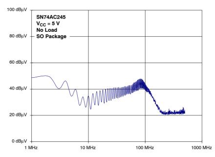
Figure 14. Frequency Spectrum of the Supply Current of an Unloaded AC Circuit (SO package)
