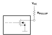
Figure 16. Open-Drain Output Principle
