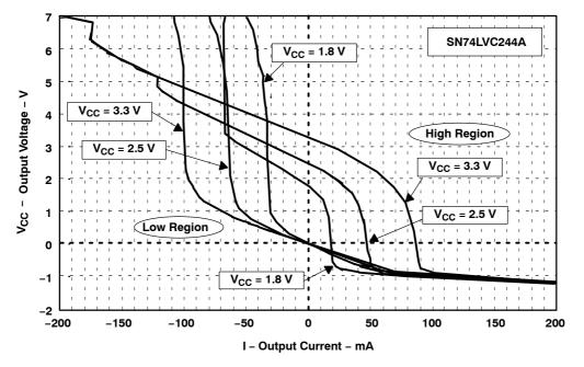
Figure 7. Output Characteristics of the LVC244 at Different Supply Voltages
