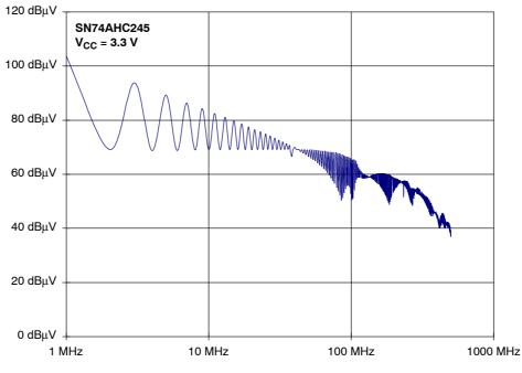
Figure 37. SN74AHC245 Spectrum of the Output Signal
