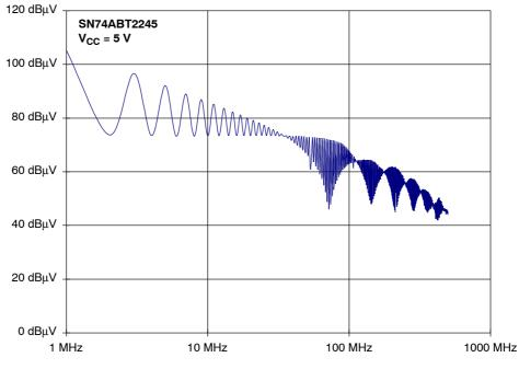
Figure 21. SN74ABT2245 Spectrum of the Output Signal
