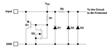
Figure 12. Two-Stage ESD-Protection Circuits
