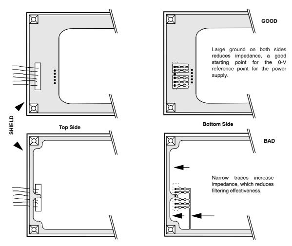
Figure 13. Mounting Filter Capacitors for External I/Os
