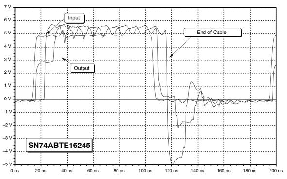
Figure 74. Output Waveforms of the SN74ABTE16245
