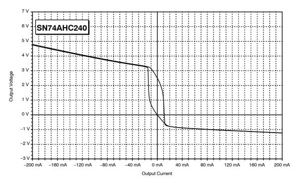
Figure 8. Output Characteristics of the SN74AHC240
