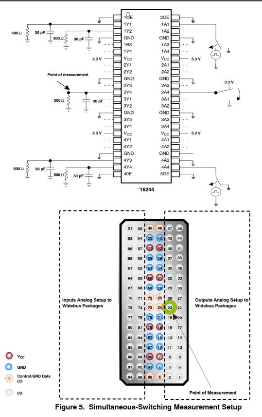
For this measurement procedure, one input is connected to a fixed low (L) state, or high (H) state, while all other inputs are switched simultaneously. The outputs of the connecting driver react to the changes in the various inputs with a certain delay, while the nonswitched output should maintain a constant low state (or high state).
