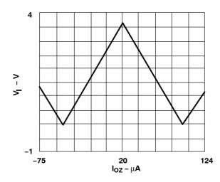
Figure 11. Power-Up/Power-Down Test With Vo = High, ALVTH16244
