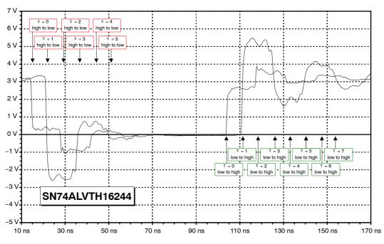
Figure 25. Signal Shape of the SN74ALVTH16244
