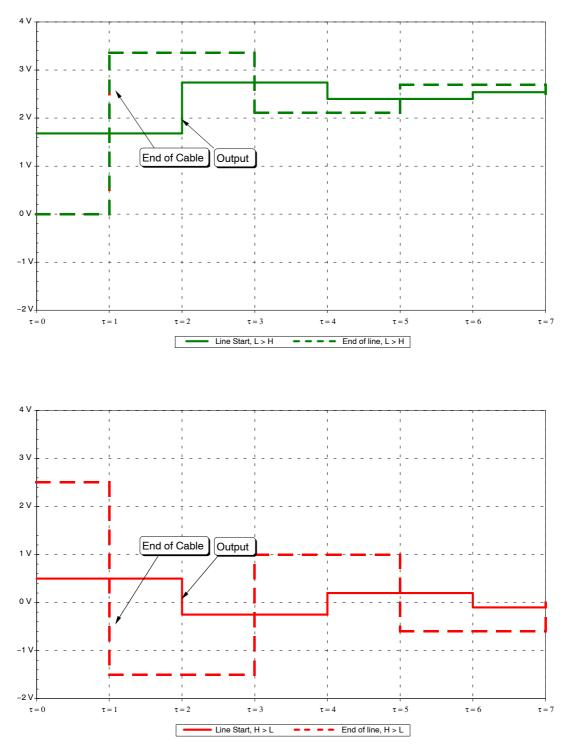
Figure 17. Diagram of Line Reflections for the SN74ALVCH16240
