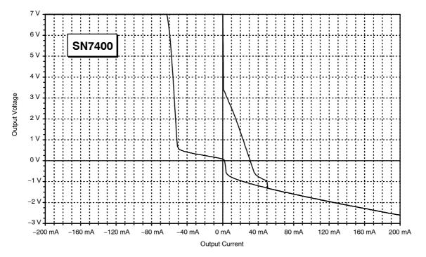
Figure 13. Output Characteristic of the SN7400
