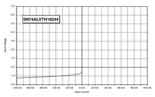
Figure 5. Input Characteristic of the SN74ALVTHxxx Series
