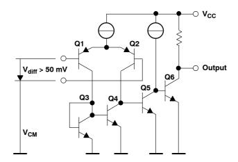
Figure 5. Simplified Circuit of a Differential Amplifier
