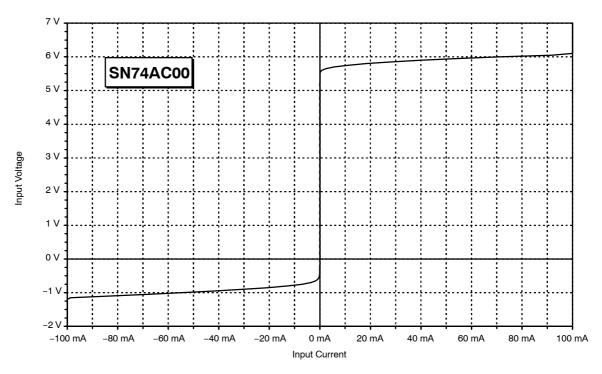
Figure 9. Input Characteristic of the SN74ACxxx Series
