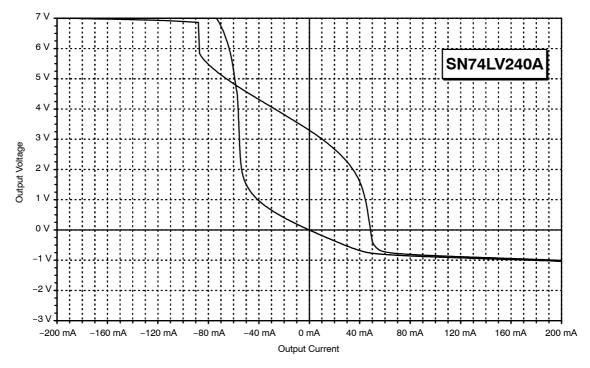
Figure 15. Output Characteristics of the SN74LV240A
