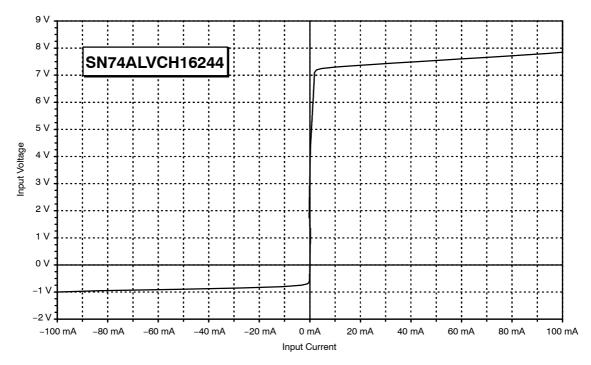
Figure 5. Input Characteristic of the SN74ALVCxxx Series
