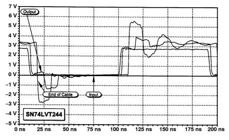
Figure 21. Waveforms on an Open-Circuit Line
