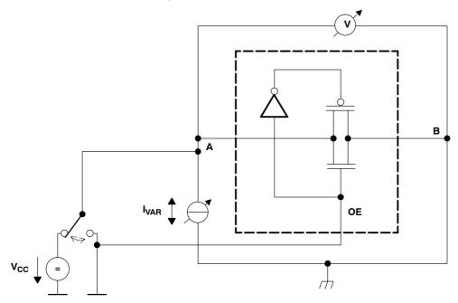
Figure 8. Setup for Measuring ron of the CBTLV3245A
