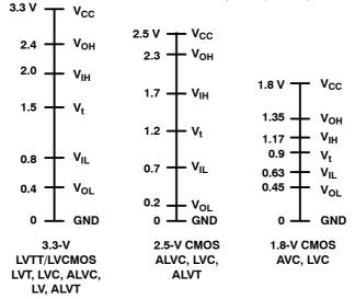
Figure 12. Comparison of Low-Voltage Switching Standards
