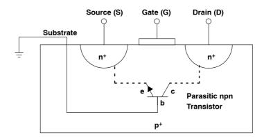
Figure 2. Cross-Sectional View of an NMOS Transistor
