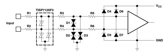
Figure 14. Protection Circuit for Extreme Requirements
