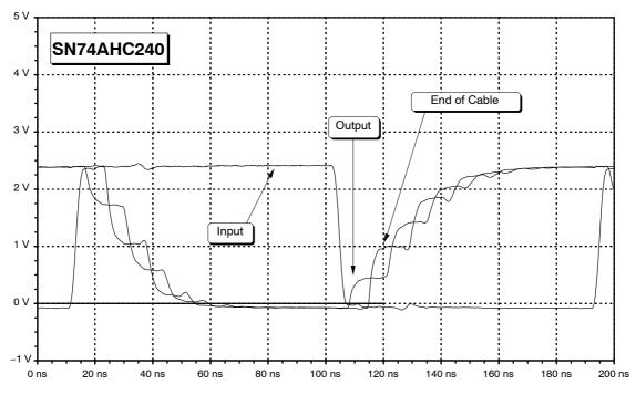
Figure 19. Output Waveforms of the SN74AHC240
