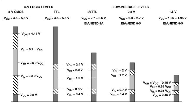
Figure 1. 5-V, 3.3-V, and 2.5-V Switching-Level Comparison
