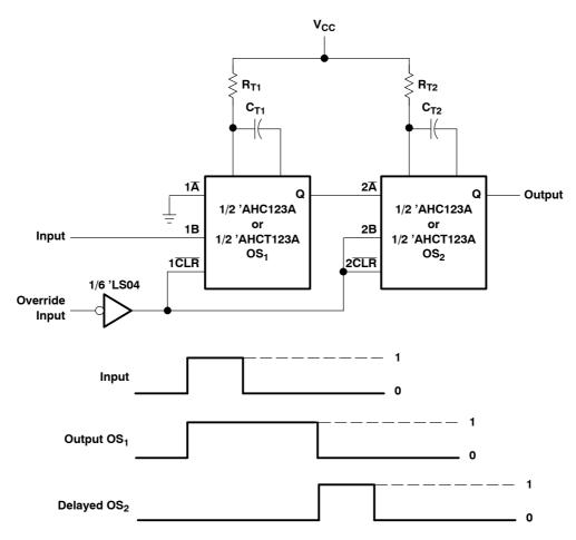
Figure 9. Delayed-Pulse Generator With Override
