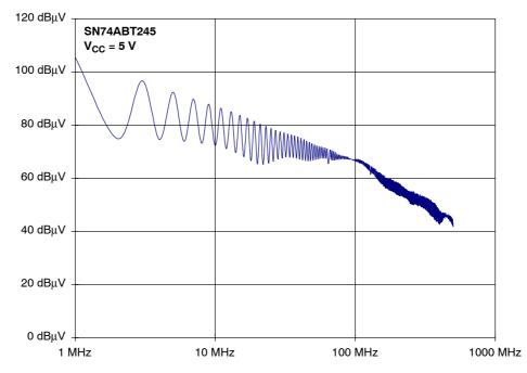
Figure 17. SN74ABT245 Spectrum of the Output Signal
