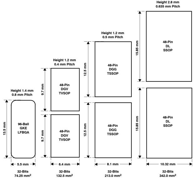
Figure 29. Space Needed for a 32-Bit Interface Using Various Packages Options
