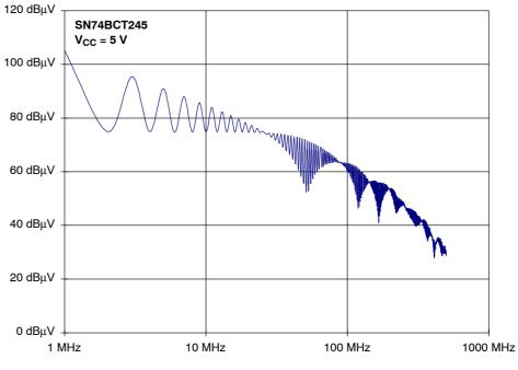
Figure 49. SN74BCT245 Spectrum of the Output Signal
