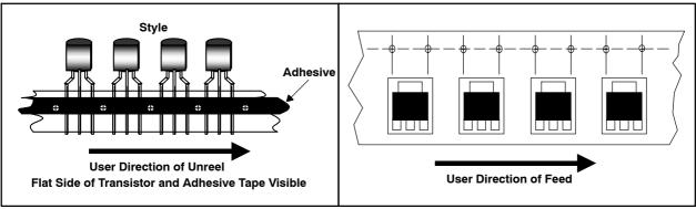
Figure 12. Typical TI Component Orientations for Tape-and-Reel Packing
