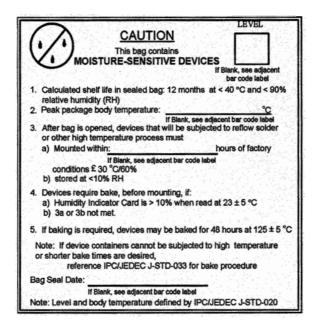
Figure 19. Moisture-Sensitivity Caution Label (Levels 2a Through 5a)
