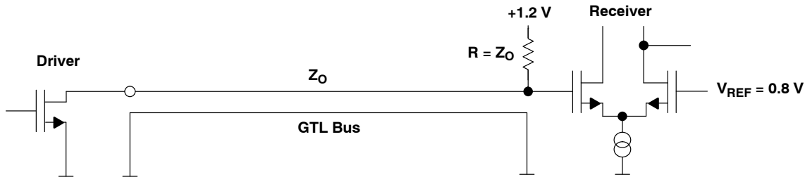
Figure 10. Circuit Concept of the GTL Bus
