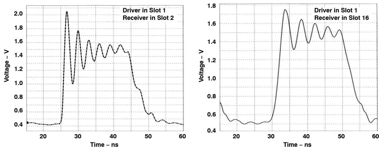
Figure 10. GTL16622A Signal Integrity (HSPICE Simulation Results)
