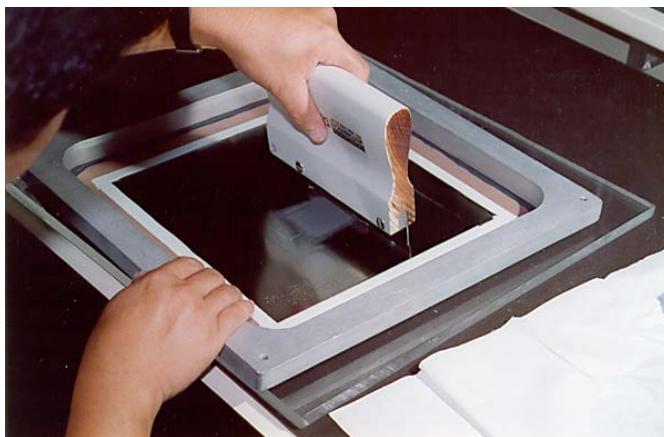
Figure 2. Solder Is Screened Onto the Ceramic Substrate
