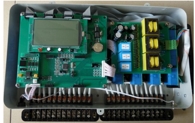
Fig. 2. Internal structure of multi-user electric energy meter.
