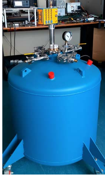
Fig. 1. Photograph of the dewar with the short cryoprobe inserted and equipment to ensure safety operation during its use.
