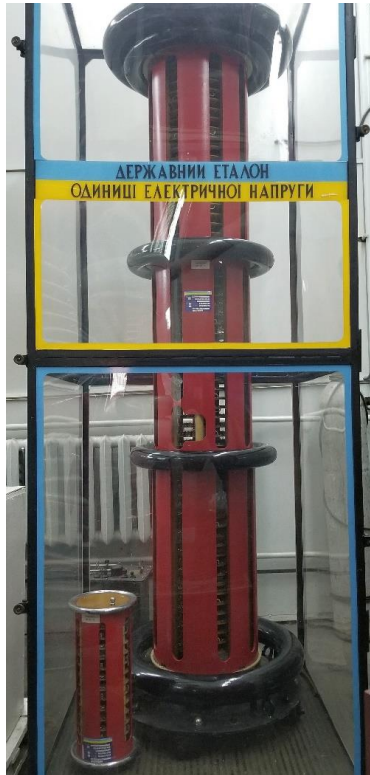
Fig. 1. The general view of National high-voltage DC standard.
