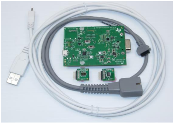
Fig. 3. AFE4403 demonstration kit.
