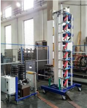
Fig. 2. LATFC's Haefely Impulse generator.
