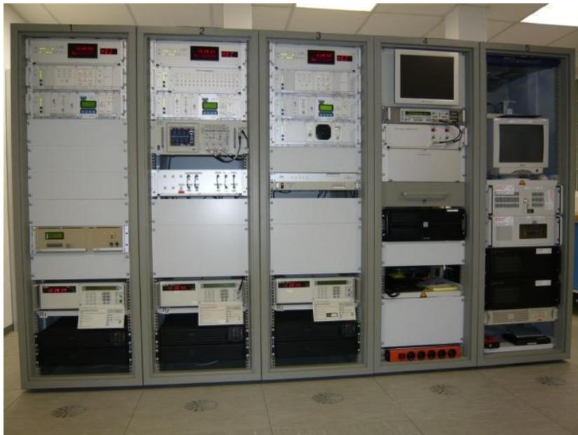
Figure 1. Electronic control unit in 2010. As a detail, one can see the three signal generators with their greenish displays and three cesium frequency standards just above the uninterruptable power supply units on the bottom.
