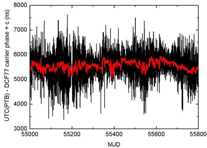
Figure 7. Carrier phase reception of DCF77 in Braunschweig: hourly data (black) and daily  $\pm 4$ -hour-averages around 12:00 UTC (red) over an extended period from MJD 55000 (2009-06-18) to MJD 55800 (2011-08-27).
