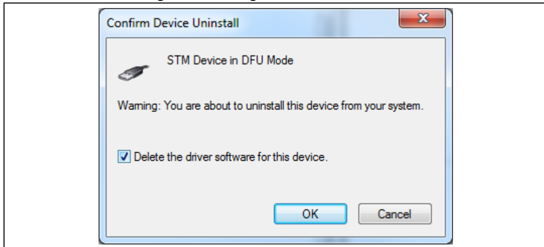
Figure 1. Deleting the old driver software
