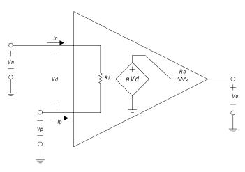
We still have the loading effects at the input and output ports as noted above. The ideal op amp model was derived to simplify circuit calculations and is commonly used by engineers in firstorder approximation calculations. The ideal model makes three simplifying assumptions:
