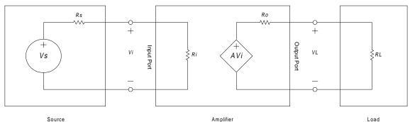
It can be seen that we have voltage divider circuits at both the input port and the output port of the amplifier. This requires us to re-calculate whenever a different source and/or load is used and complicates circuit calculations.
