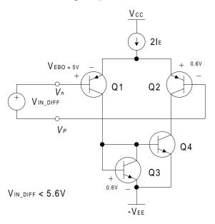
Some devices have protection built into them, and the current into the input needs to be limited. Normally, differential input mode voltage limit is not a design issue.
