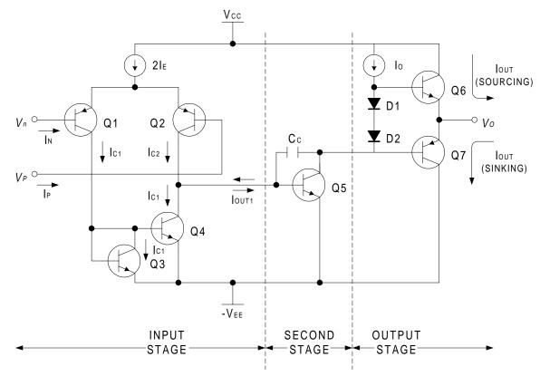
Although simplified, this circuit contains the three basic elements normally found in op amps:
