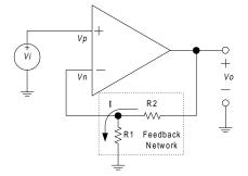
To understand this circuit we must derive a relationship between the input voltage,  $V_i$ , and the output voltage,  $V_O$ .
