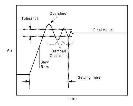
Settling time is a design issue in data acquisition circuits when signals are changing rapidly. An example is when using an op amp following a multiplexer to buffer the input to an analog to digital converter. Step changes can occur at the input to the op amp when the multiplexer changes channels. The output of the op amp must settle to within a certain tolerance before the analog to digital converter samples the signal.
