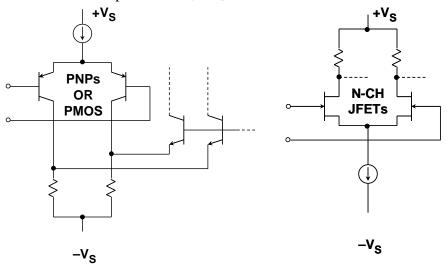
Figure 4: PNP/PMOS or N-Channel JFET Stages Allow CM Inputs to the Negative Rail
