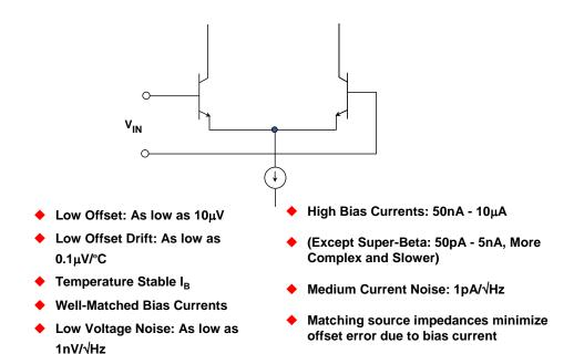
Figure 2: A Bipolar Transistor Input Stage
