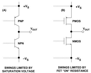
Figure 7: "Almost" Rail-To-Rail Output Structures
