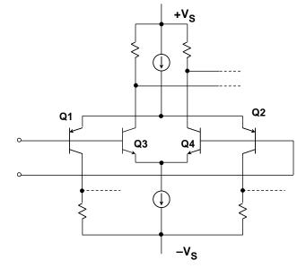
Figure 5: A True Rail-To-Rail Bipolar Transistor Input Stage
