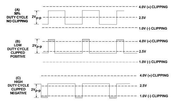
Figure 9: Headroom Issues with Single Supply Biasing
